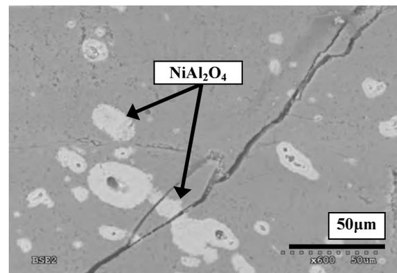
Fig. 6. Example crack propagation observed in spinel phase  $NiAl_2O_4$  particle
