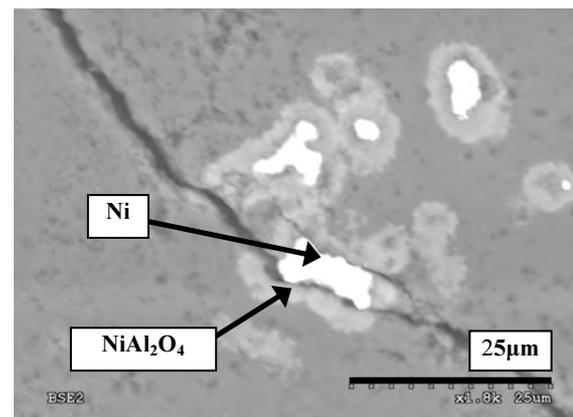
Fig. 7. Example crack propagation observed on Ni/ $NiAl_2O_4$  particles border
