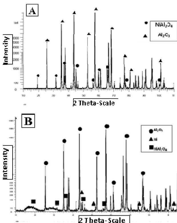
Fig. 2. Phase analysis of Al<sub>2</sub>O<sub>3</sub>+1% vol. Ni composite: A) made on sample surface (AREA I), B) made on cross-sectional sample (AREA II)
