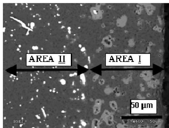
Fig. 1. SEM photo of cross-section of  $\text{Al}_2\text{O}_3+3\% \text{ Ni}$  composite
