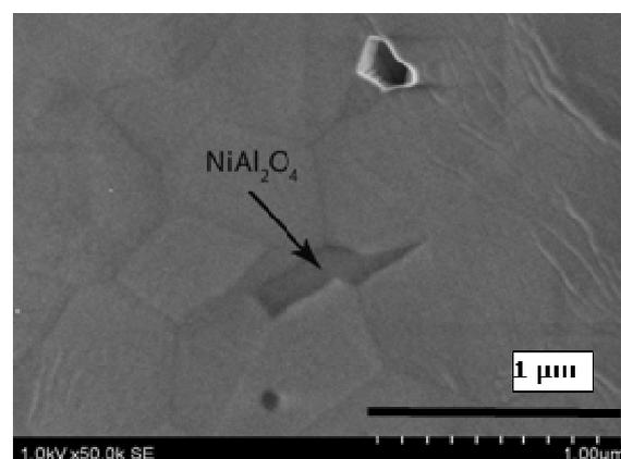
Fig. 3. Transmission electron microscope images of Al<sub>2</sub>O<sub>3</sub>+1% vol. Ni composite with spinel phase
