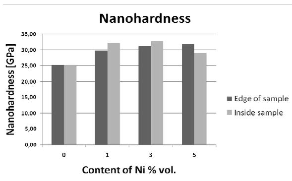
Fig. 4. Nanohardness  $Al_2O_3+x\% Ni$  composites
