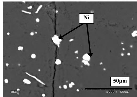
Fig. 5. Deflection of crack coming out of corners of Vickers indentation
