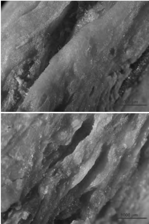
Fig. 3. Cracking of cement mass
