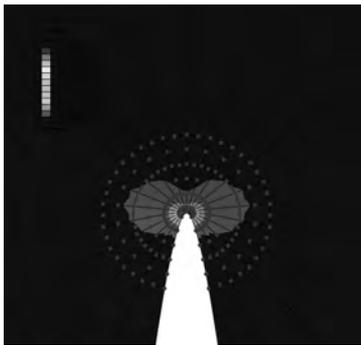
Fig. 7. Distribution of stress according to H-M-H hypothesis in fourth circle at moment of crack initiation
