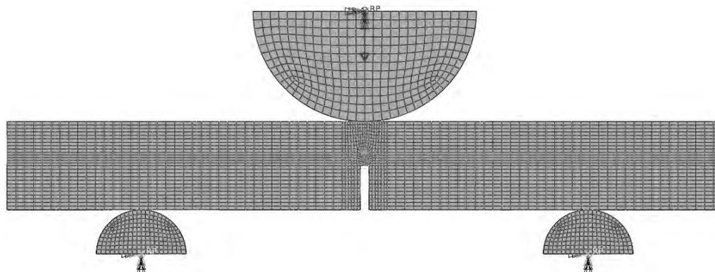
Fig. 5. General view of calculation model for SENB type sample for crack resistance testing
