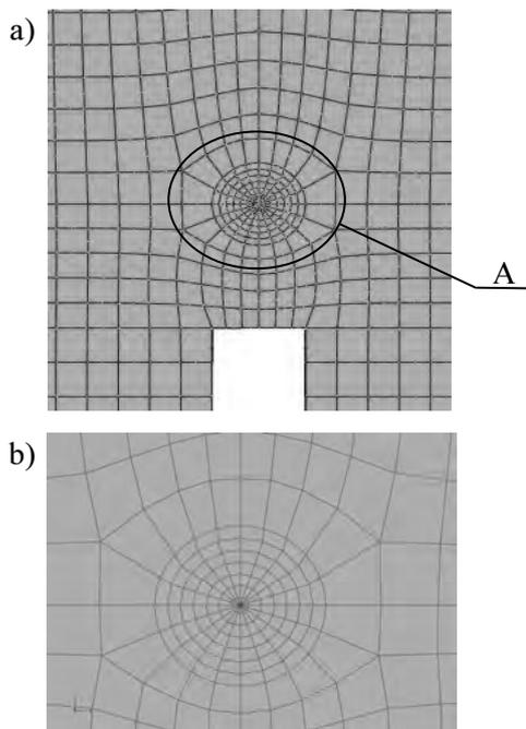
Fig. 6. Grid of finite elements near crack peak: a) general view, b) detail A
