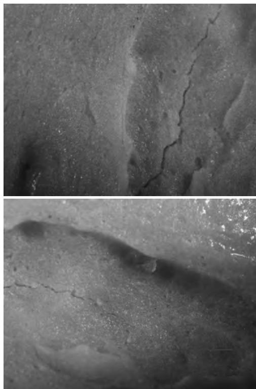
Fig. 1. Microcracks observed in PMMA directly after polymerization process
