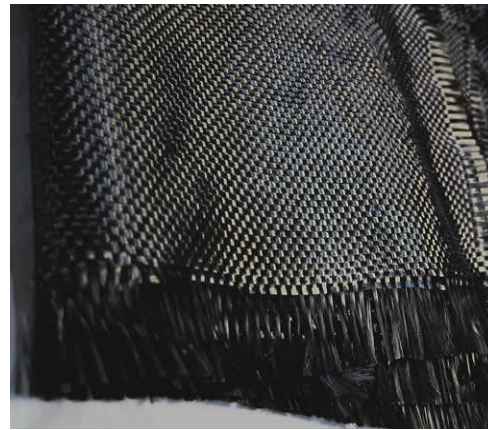
Fig. 2. CF072 - carbon 300 g/m 2 of plain type: 1/1 weave, from Suretexcomp company - continuous roving, plain weave, no magnification
