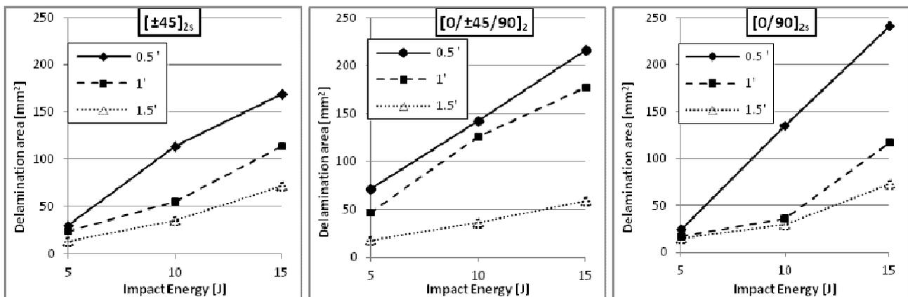
Fig. 4. Relationship between area of delamination and impact energy for analysed laminates
