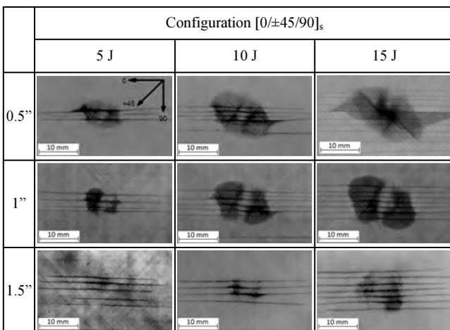
Fig. 2. Typical failure of GFRP plates with  $[0/\pm 45/90]_s$  configuration
