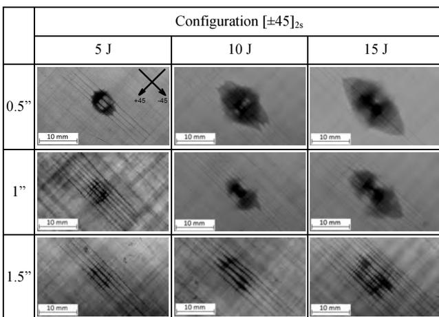
Fig. 1. Typical failure of GFRP plates with  $[\pm 45]_{2s}$  configuration
