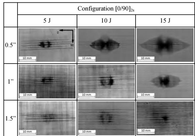
Fig. 3. Typical failure of GFRP plates with  $[0/90]_{2s}$  configuration
