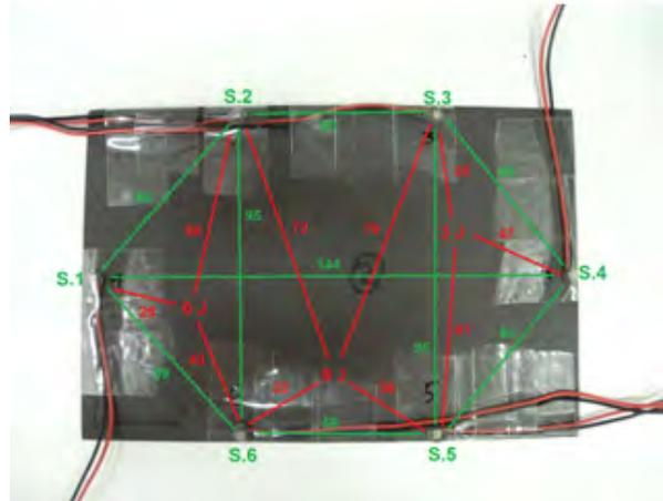
Fig. 2. PZT network on CFRP specimen number 1 (dimensions are in millimeters)
