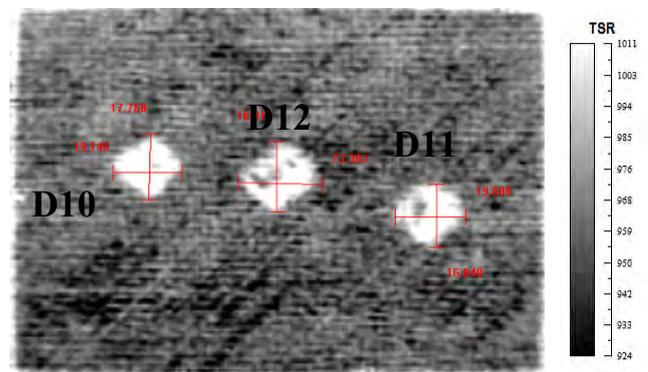
Fig. 7. Test results for CFRP specimen number 2 after impact - thermography method
