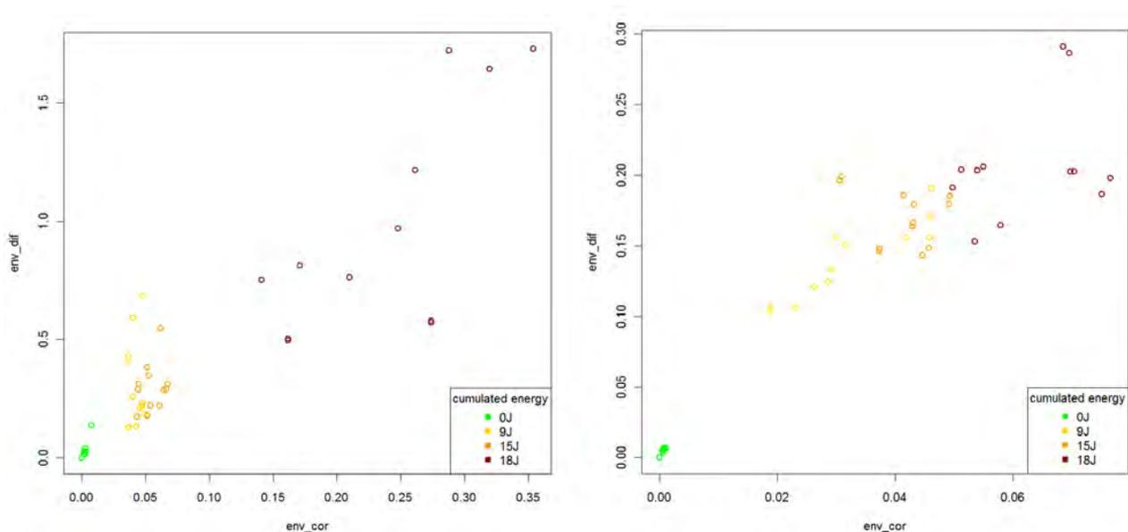
Fig. 12. Average damage indicators for CFRP specimen: number 1 (left graph) and number 2 (right graph)
