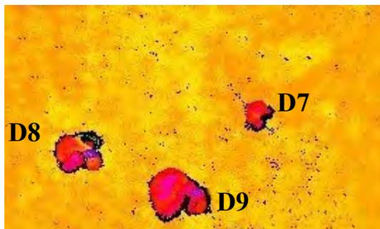
Fig. 10. Test results for CFRP specimen number 1 after impact - UT method
