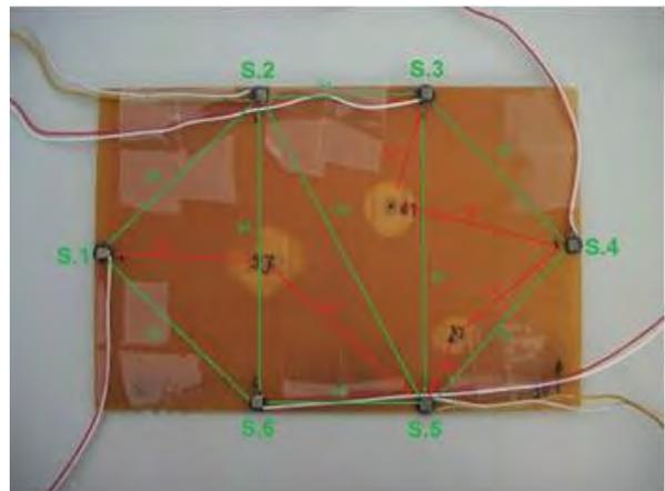
Fig. 3. PZT network on GFRP specimen number (dimensions are in millimeters)
