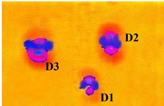
Fig. 8. Test results for GFRP specimen number 1 after impact - UT method
