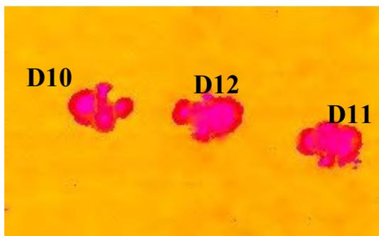
Fig. 11. Test results for CFRP specimen number 2 after impact - UT method
