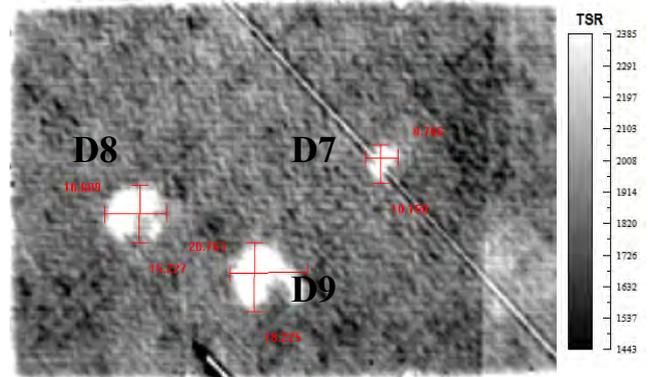
Fig. 6. Test results for CFRP specimen number 1 after impact - thermography method
