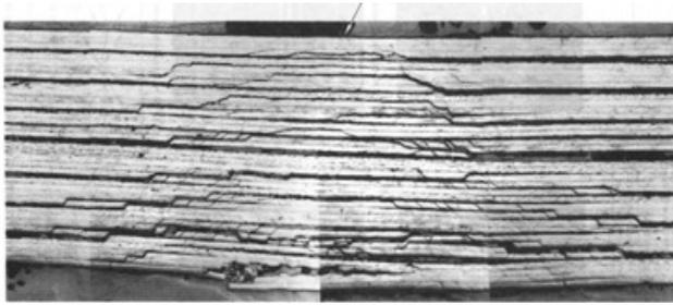
Fig. 1. BVID in CFRP composite structure [2]
