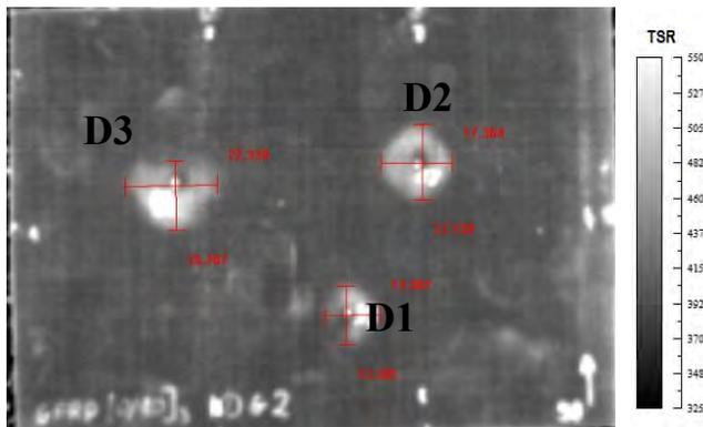
Fig. 4. Test results for GFRP specimen number 1 after impact - thermography method
