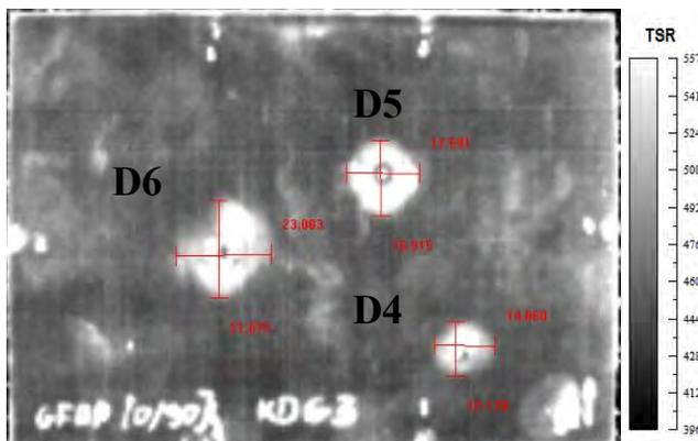
Fig. 5. Test results for GFRP specimen number 2 after impact - thermography method
