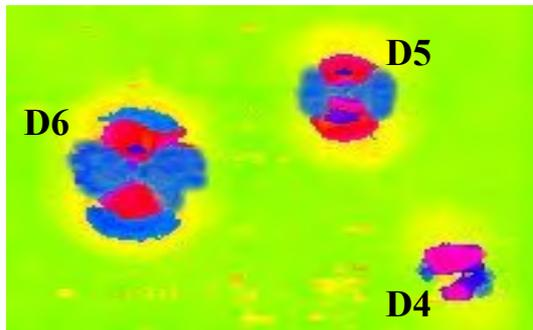
Fig. 9. Test results for GFRP specimen number 2 after impact - UT method
