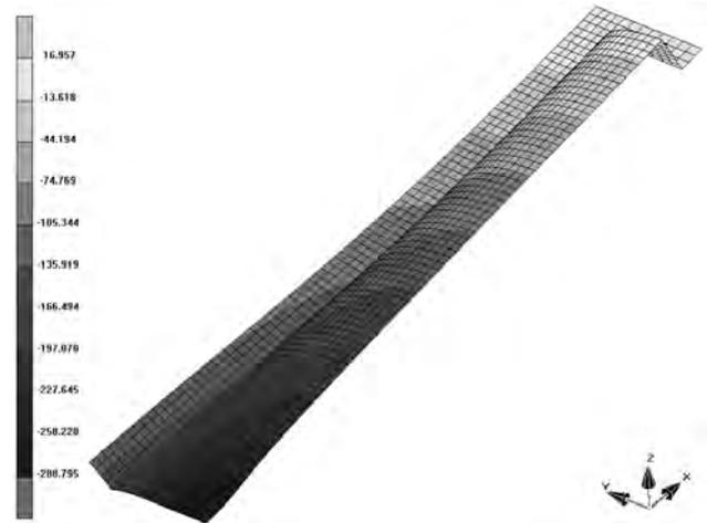
Fig. 7. Vertical displacements contour  $z$ [mm] for  $s = 280$  mm
