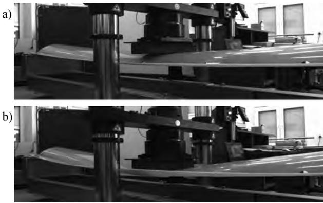
Fig. 3. Segment bending test at selected punch positions: a)  $s = 160$  mm;
