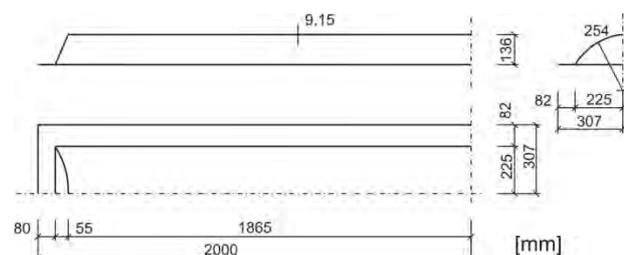
Fig. 1. Overall dimensions of composite segment quarter
