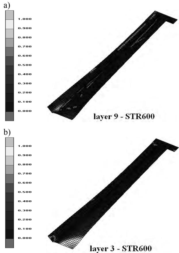
Fig. 8. Contours for selected failure indices for  $s = 280$  mm: a) F11 in layer 9; b) F14 in layer 3
