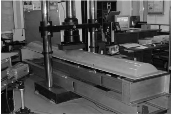
Fig. 2. Test stand for composite segment bending test
