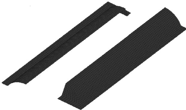
Fig. 4. FEM numerical model of composite segment quarter
