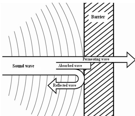
Fig. 1. Sound wave propagation [4]
