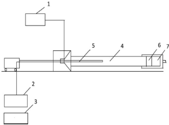
Fig. 3. Measuring path for determining sound absorption coefficient [10]: 1 - acoustic generator, 2 - measuring amplifier, 3 - filter system, 4 - Kundt's tube, 5 - microphone probe, 6 - tested material, 7 - sealing disc
