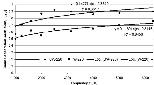
Fig. 4. Dependence of sound absorption coefficient on frequency
