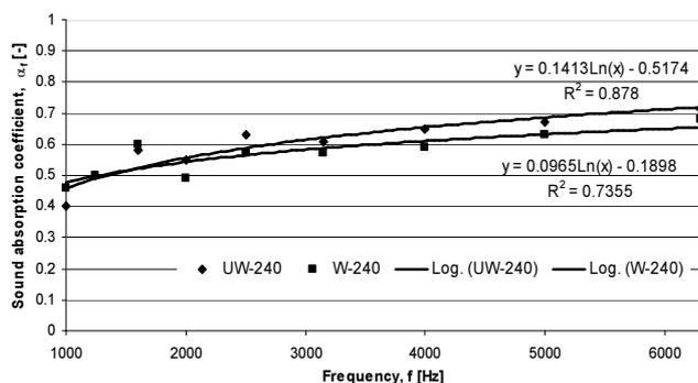
Fig. 5. Dependence of sound absorption coefficient on frequency
