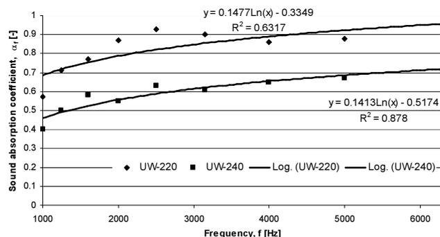
Fig. 6. Dependence of sound absorption coefficient on frequency
