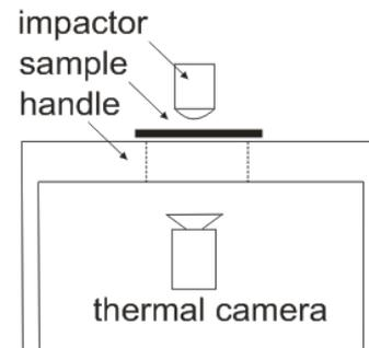
Fig. 1. Stand for low-velocity impact recording by using thermal camera
