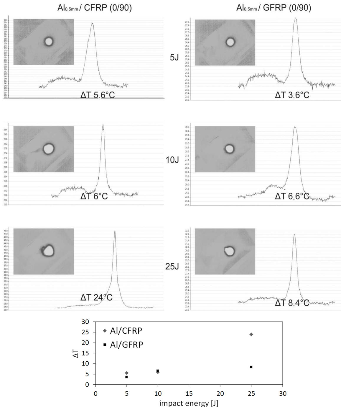
Fig. 2. Profile and growth value of temperature in impact area of FML depending on impact energy
