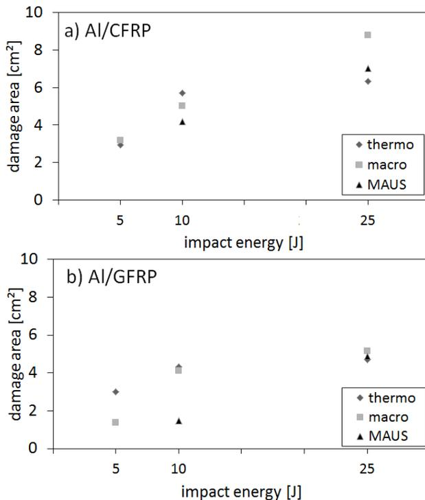
Fig. 3. FML damage area (a - Al/CFRP, b - Al/GFRP) measured with: thermography, ultrasonic and visual methods
