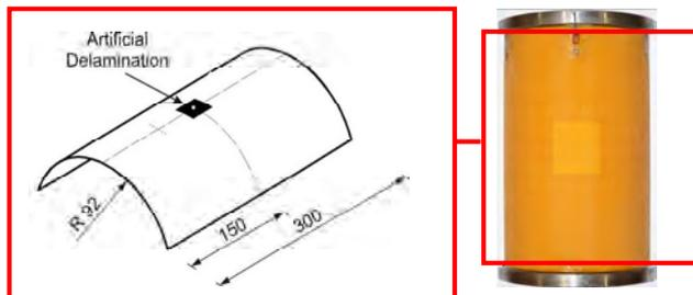
Fig. 3. Geometry of cylindrical composite shell
