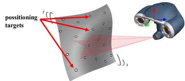
Fig. 1. Data acquisition in 3D scanning process [10]
