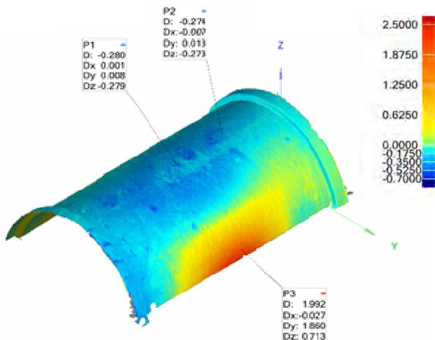
Fig. 8. Comparison of 3D deviation of deformed composite structure
