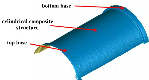
Fig. 4. Virtual model of scanning surface
