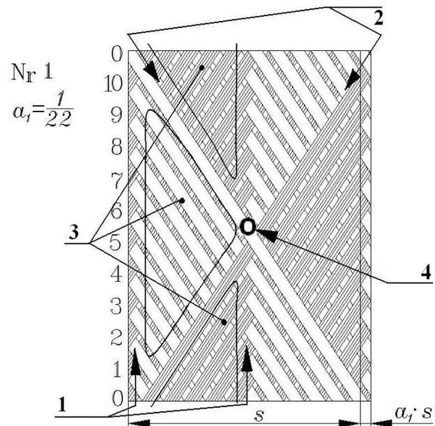
Fig. 2.  $N_r1$  mosaic pattern scheme with characteristic areas: 1 - crossover lines (circumferential band), 2 - fibre undulation line (helical band), 3 - areas without crossovers (undulations), 4 - central point, s - winding lead,  $a_1$  - coefficient
