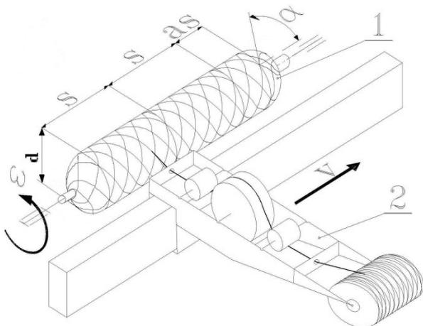
Fig. 1. Filament winding scheme: 1 - mandrel, 2 - support, s - winding lead, a - coefficient, a  $\epsilon(0,1)$
