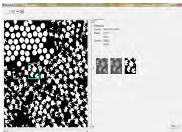
Fig. 3. Window of SAO software for determining composite material component fractions. In upper left corner of processed picture, effect of manual carbon fiber marking is presented. Magnification 500x
