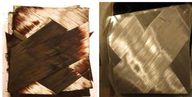
Fig. 4. Examples of specimens with carbon and glass (hybrid) fibers after calcination
