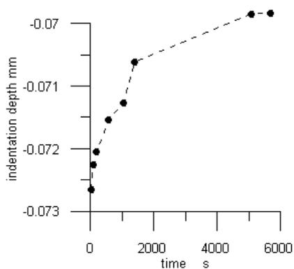
Rys. 7. Variation of dent depth with time for dent resulting from 9 J impact
