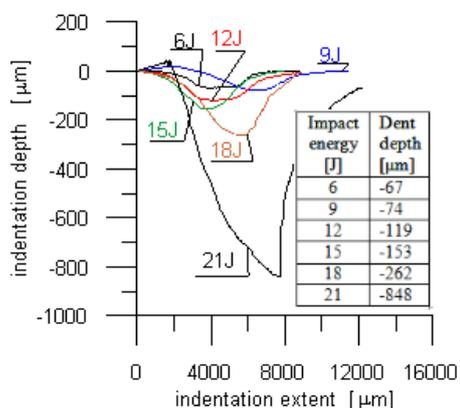
Rys. 6. Indentation depths and profiles
