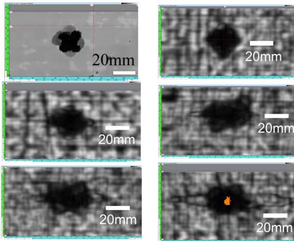
Rys. 9. C-scans of impact damage areas
