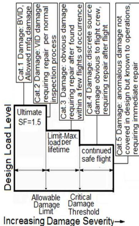
Rys. 1. Regulatory airworthiness requirements relating damage or defect size to load capacity of structure. Precise definition of damage categories can be found in [1]
