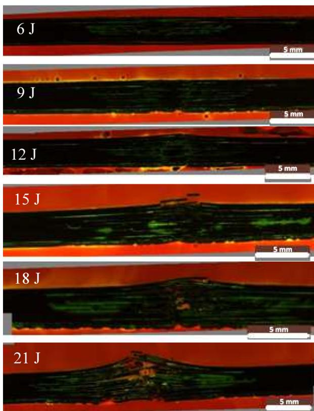
Rys. 10. Fractography of impact damages. Sectioning along major ellipse axis. Length of white line section corresponds to 5 mm
