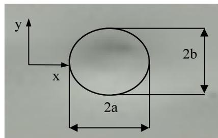
Rys. 8. Described ellipse of impact imprint. Usually for quasi isotropic laminate  $a \approx b \approx R$  [3]
