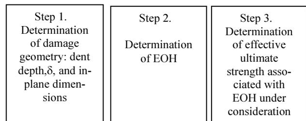
Rys. 2. General algorithm of simplified procedure to determine ultimate strength that makes provision for adverse effect of BVID
