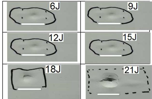
Rys. 4. Impact imprints shown to inspectors. Length of white line section corresponds to 2 mm
