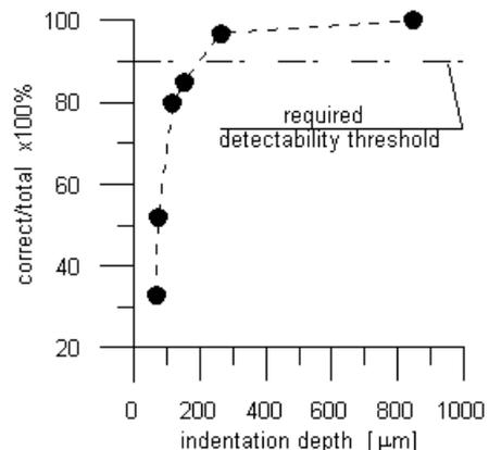
Rys. 5. Damage detectability in terms of correct over total answers ratio versus indentation depth. Required detectability threshold of 90% is acceptable by aviation authorities
