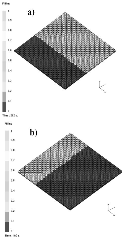
Fig. 5. Screens from PAM-RTM program. Exemplary simulation of filling plain-woven fabric preform: a) direction 2 (Y), b) direction 1 (X)
