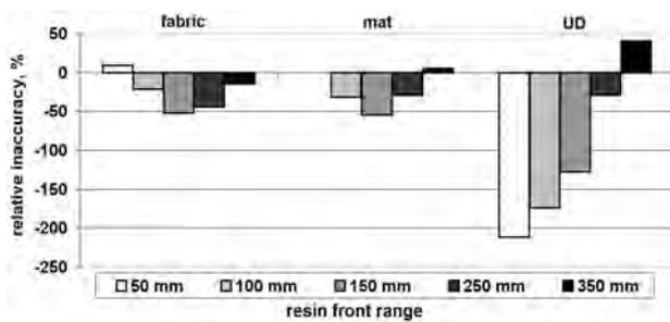
Fig. 8. Relative inaccuracy of simulation time results against experimental (approximation) time results. Diagonal resin flow, measurement along diagonal of preform. Negative values mean that real process runs faster for given type of preform in particular phase
