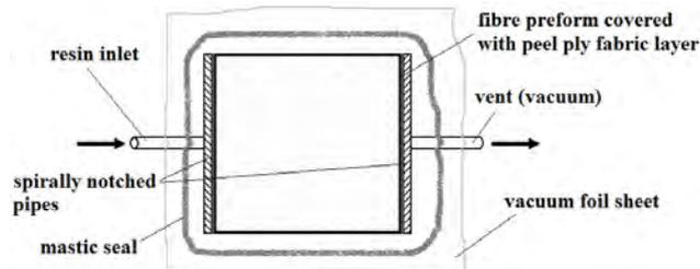
Fig. 2. Diagram of stand for VARI processes performed within study
