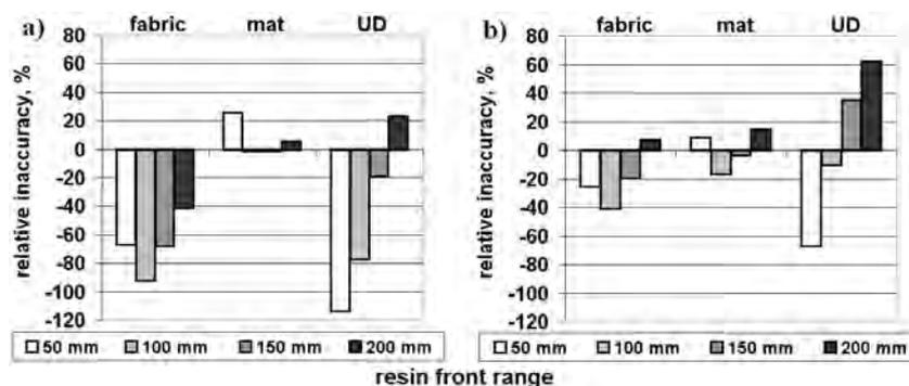
Fig. 9. Relative inaccuracy of simulation time results against experimental (approximation) time results. Diagonal resin flow, measurement along directions 1 (a) and 2 (b) of preform. Negative values mean that real process runs faster for given type of preform in particular phase
