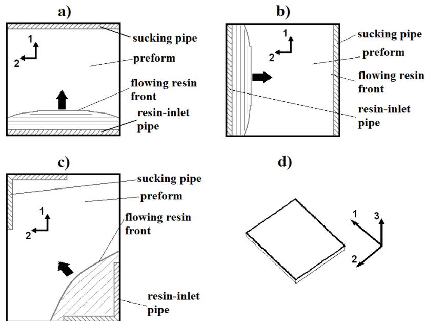
Fig. 3. Diagrams of resin flow through preforms applied in study: a), b) linear flow, c) diagonal flow, d) indications of directions within preform (directions 1 and 2 are consistent with those in Fig. 1)
