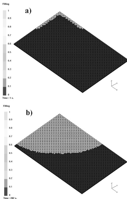
Fig. 7. Screens from PAM-RTM program. Exemplary simulation of filling plain-woven fabric preform in diagonal direction: a) initial phase, b) advanced phase
