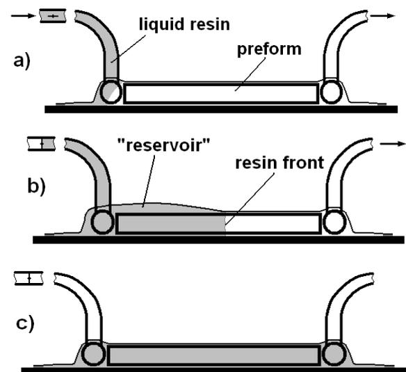
Fig. 10. Stages of VARI process: a) initial stage, b) intermediate stage - creation of "reservoir", c) end of process - preform completely filled with resin
