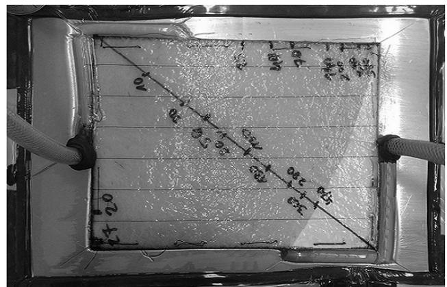
Fig. 6. Exemplary preform (chopped strand mat) processed by VARI, diagonal resin flow
