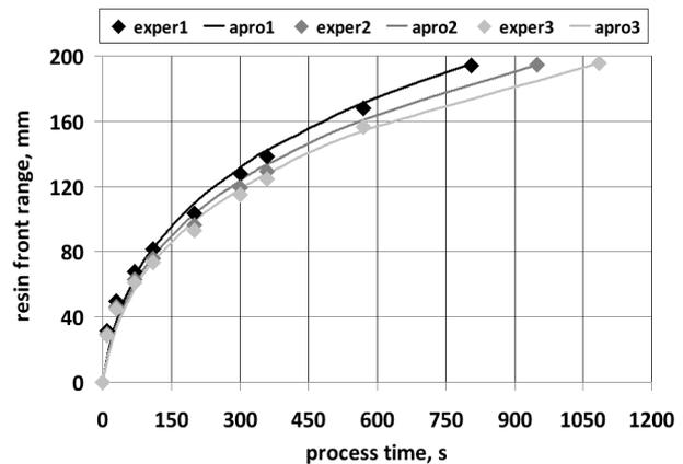
Fig. 4. Exemplary set of *resin front range vs. process time* relations and corresponding approximation curves: plain weave fabric preform, resin flow in direction 1
