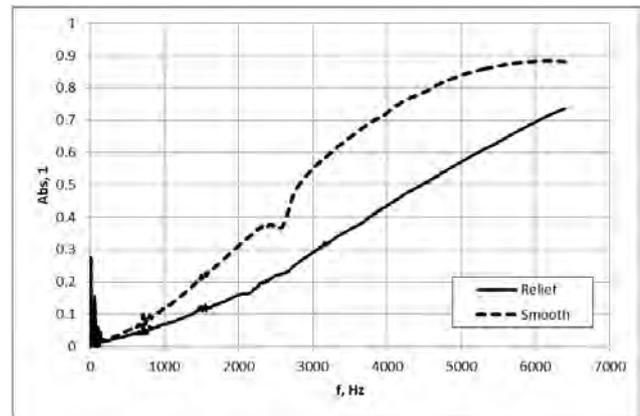
Fig. 9. Sound absorption coefficient of composite 7 (smooth-relief,  $\phi$  17 mm)
