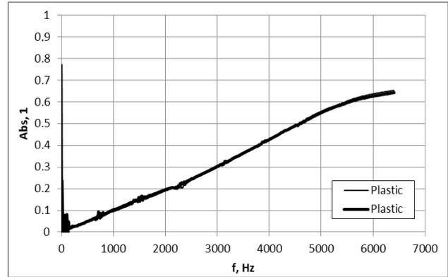
Fig. 3. Sound absorption coefficient of composite 1 (plastic-plastic)
