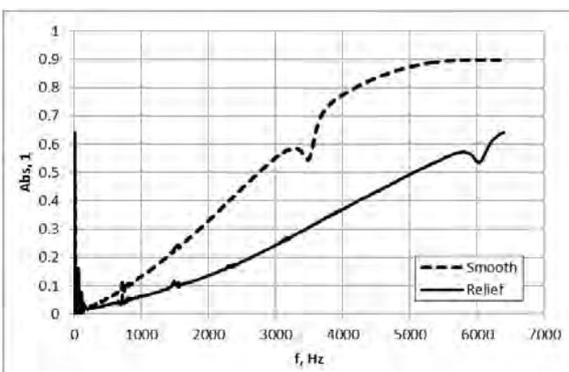
Fig. 8. Sound absorption coefficient of composite 6 (smooth-relief,  $\phi$  13 mm)
