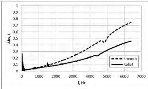
Fig. 6. Sound absorption coefficient of composite 4 (smooth-relief,  $\phi$  5 mm)
