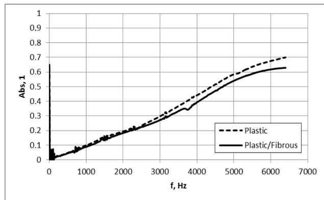
Fig. 4. Sound absorption coefficient of composite 2 (plastic/fibrous-plastic)
