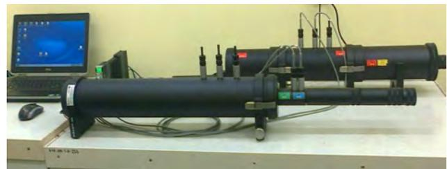
Fig. 1. Test set-up with Kundt tube
