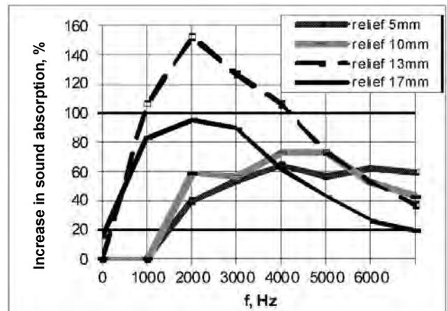
Fig. 10. Increase in sound absorption for composite side with smooth surface in relation to relief side
