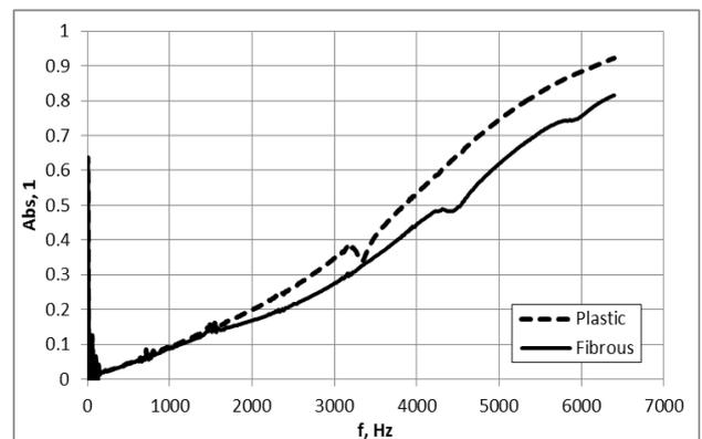
Fig. 5. Sound absorption coefficient of composite 3 (fibrous-plastic)
