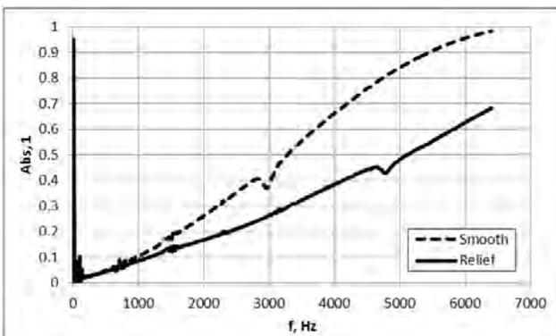
Fig. 7. Sound absorption coefficient of composite 5 (smooth-relief,  $\phi$  10 mm)
