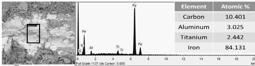
Fig. 5. Chemical analysis of third body on working surface
