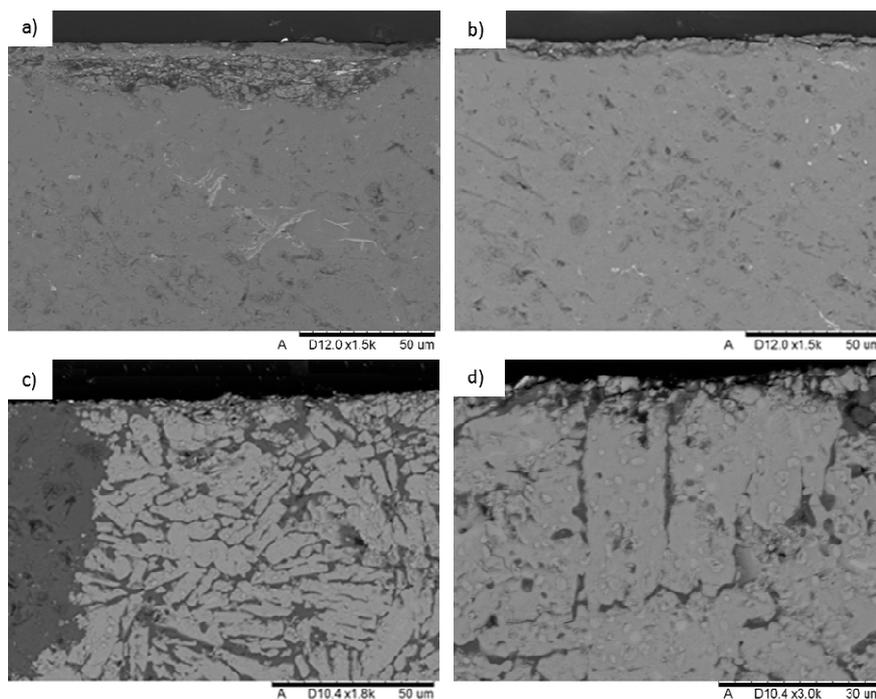
Fig. 8. SEM micrographs of cross sections of samples: a) Al-Si matrix - debris, b) Al-Si matrix - separated layer after crack, c) MAX phase + Al-Si composite material, d) MAX phase + Al-Si composite material - degradation of MAX phase platelets
