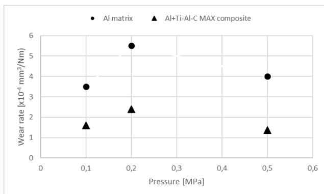
Fig. 6. Wear rate in function of applied load
