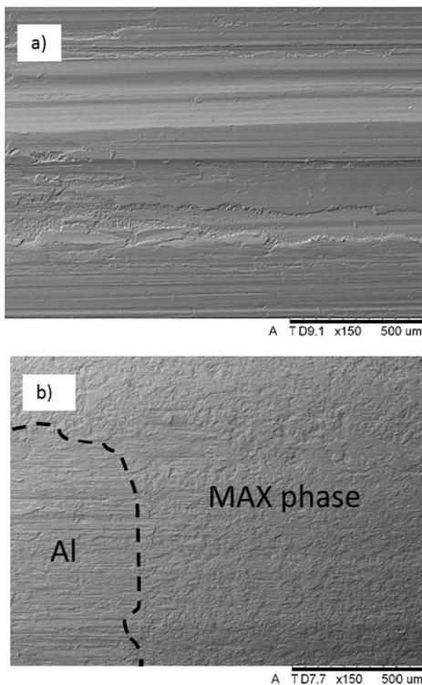
Fig. 3. Topography of working surfaces: a) Al-Si matrix, b) MAX phase + Al-Si composite material
