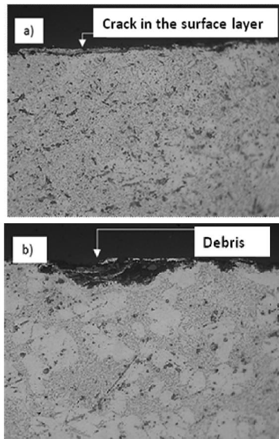
Fig. 7. View of cross sections of samples: a) Al-Si matrix, b) MAX phase + Al-Si composite material
