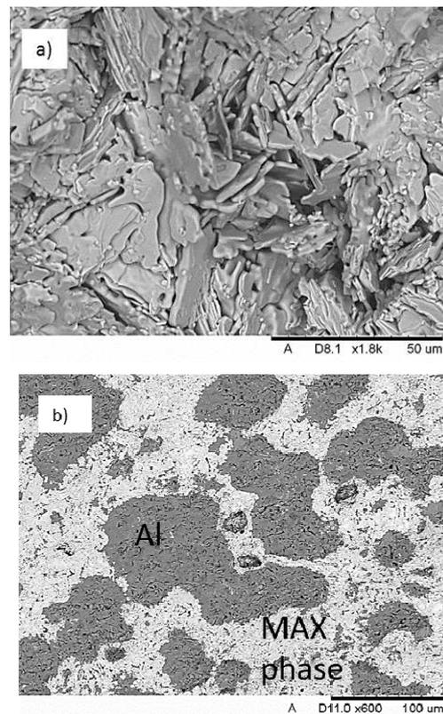
Fig. 1. View of microstructure of manufactured samples: a) MAX phase reinforcement, b) MAX phase ( $\text{Ti}_2\text{AlC}$  i  $\text{Ti}_3\text{AlC}_2$ ) + Al-Si composite material
