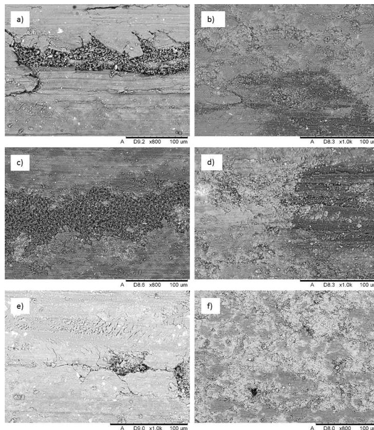
Fig. 4. Comparison of working surfaces for different loads: a) 0.1 MPa, matrix, b) 0.1 MPa, composite, c) 0.2 MPa, matrix, d) 0.2 MPa, composite, e) 0.5 MPa, matrix, f) 0.5 MPa, composite
