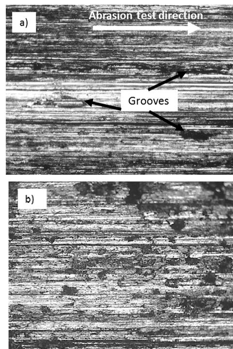
Fig. 2. View of working surfaces: a) Al-Si matrix, b) MAX phase + Al-Si composite material
