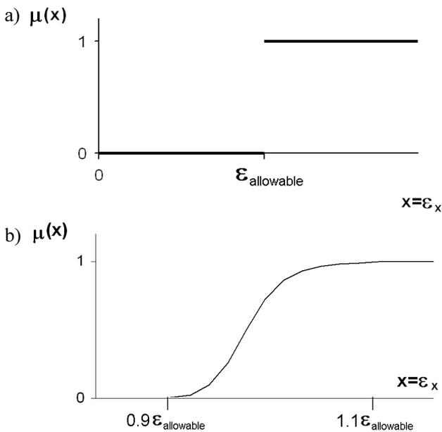
Fig. 1. Representation of term “failure under tension”: a) crisp set, b) fuzzy set
