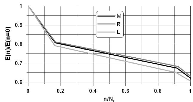
Fig. 4. Degradation of laminate (glass fiber/epoxy resin) stiffness vs. number of cycles (mean values - M, upper - R and lower - L bounds, respectively)
