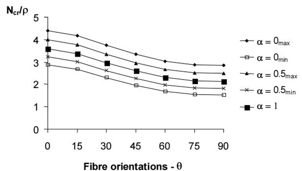
Fig. 6. Distributions of buckling loads for compressed angle-ply plates
