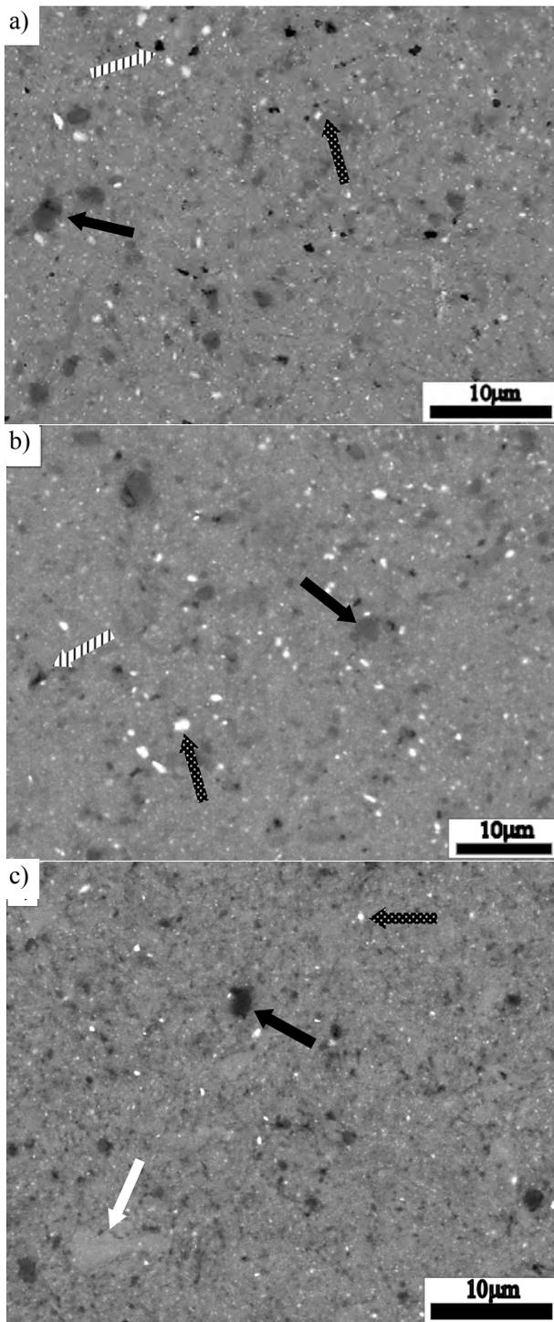
Fig. 3. SEM (BSE) micrographs of hot pressed composite powders with 10 wt.% of: a) -325 mesh AlN, b)  $\sim 1 \mu\text{m}$  AlN and c) submicron AlN; arrows designation: black - AlN particles, white - recrystallized Al, striped - pores, dotted - intermetallic precipitates
