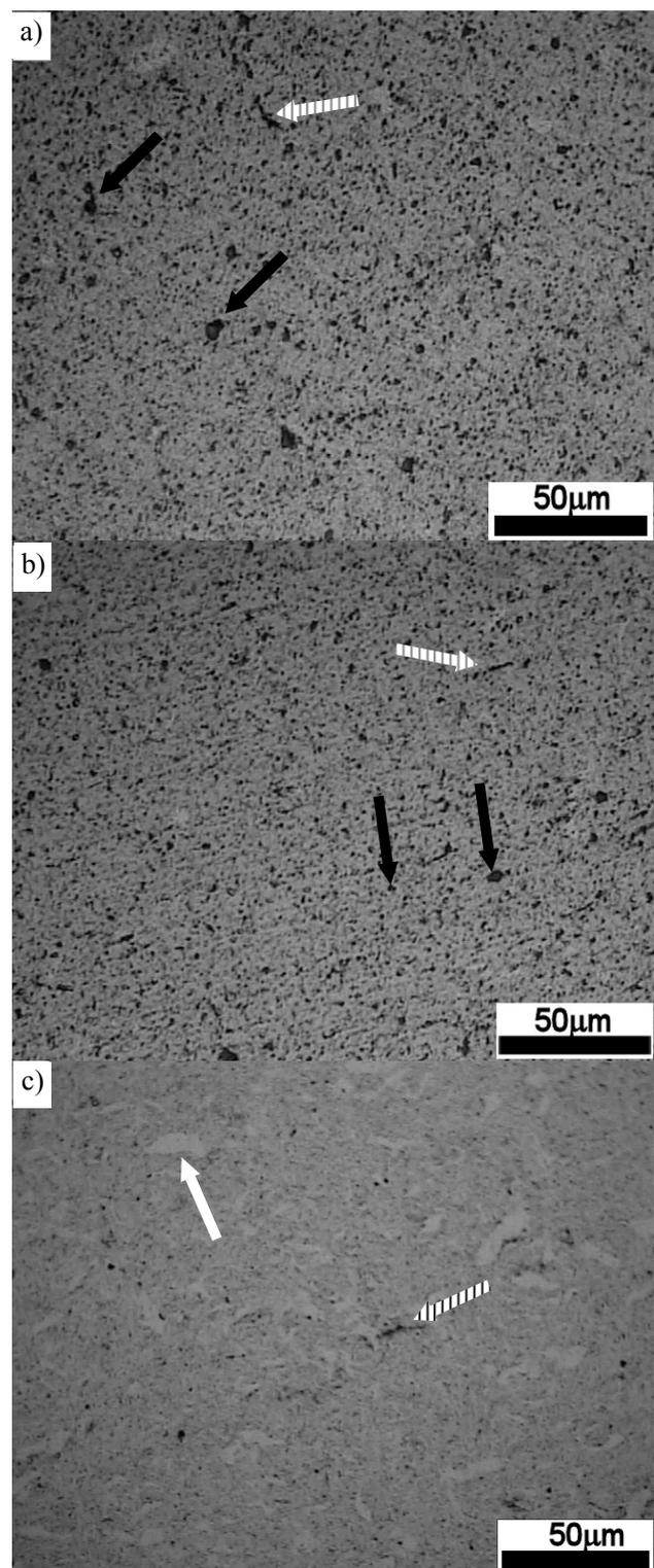
Fig. 2. Optical microstructure of hot pressed composite powders with 10 wt.% of: a) -325 mesh AlN, b)  $\sim 1 \mu\text{m}$  AlN and c) submicron AlN; arrows designation: black - AlN particles, white - recrystallized Al, striped - pores
