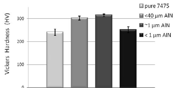
Fig. 4. Vickers hardness of 7475/AlN<sub>10%</sub> composites
