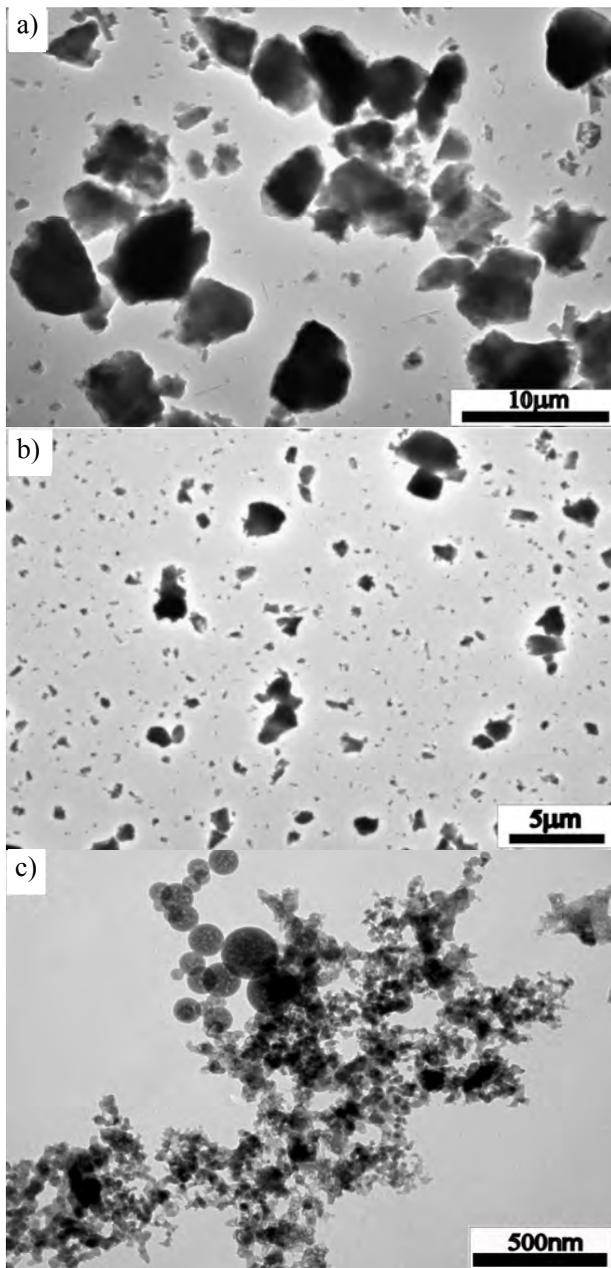
Fig. 1. Bright-field TEM micrographs of AlN powders: a) -325 mesh AlN, b)  $\sim 1 \mu\text{m}$  AlN and c) submicron AlN
