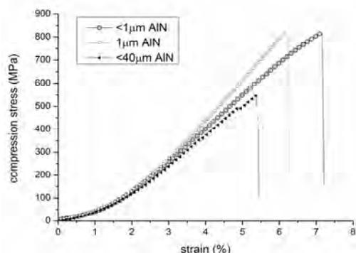
Fig. 5. Compression curve of 7475/AlN<sub>10%</sub> composites
