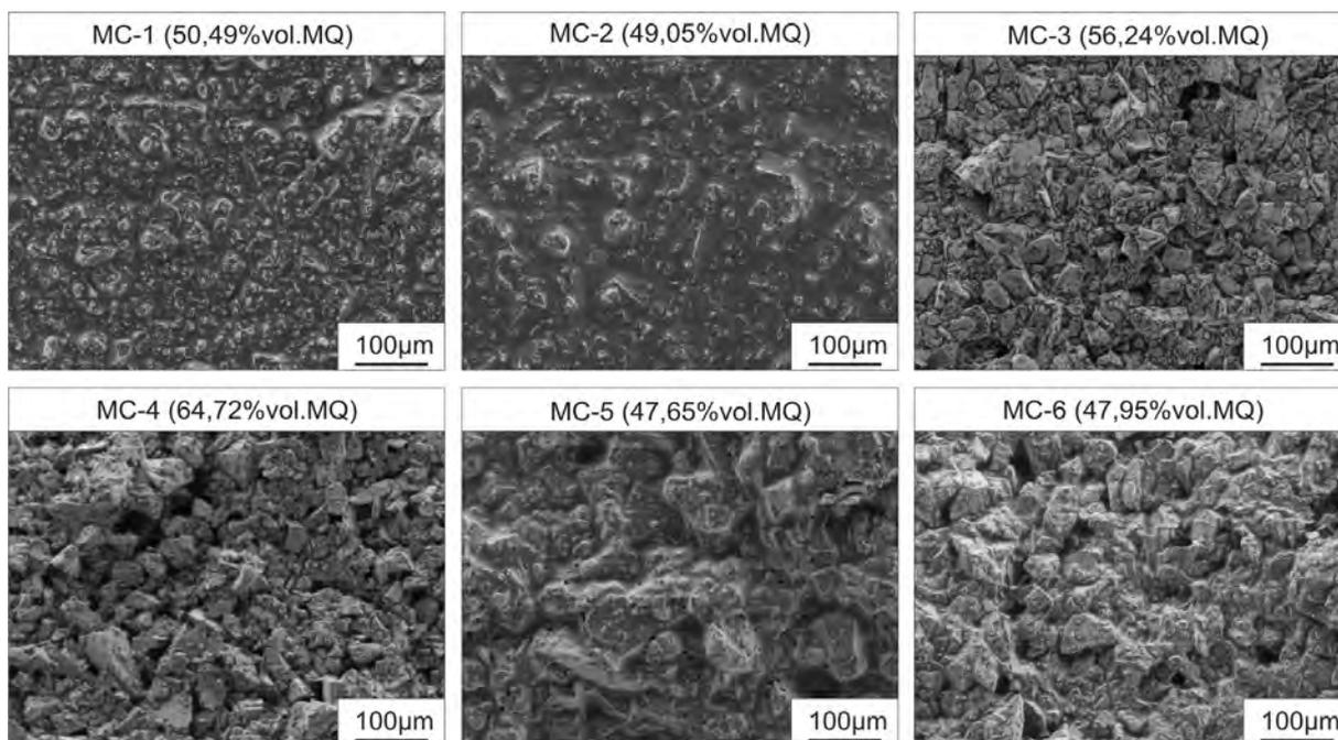
Fig. 4. Morphology of rough surfaces of composite magnetic foils
