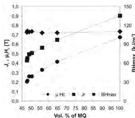
Fig. 3. Remanence ( $J_r$ ), coercivity ( $\mu_0H_c$ ) and maximum energy product (BH)max versus MQ powder content for magnetic composite foils
