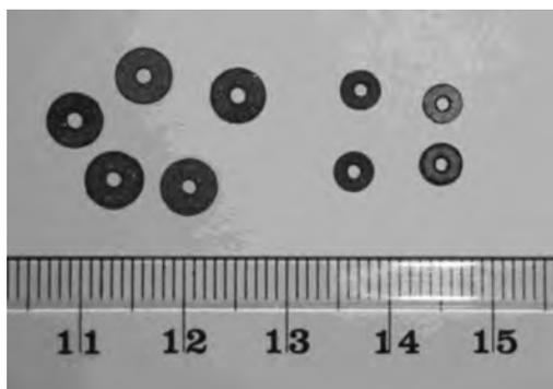
Fig. 6. Composite magnetic discs rotors for miniature electric motors
