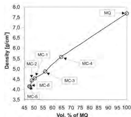
Fig. 1. Density versus MQ powder content for composite magnetic foils
