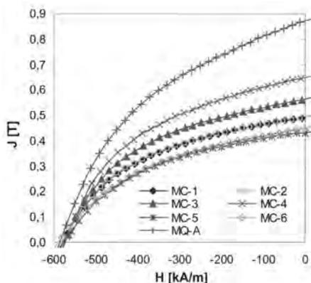
Fig. 2. Demagnetization curves for composite magnetic foils
