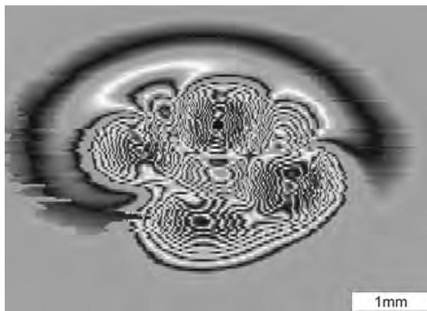
Fig. 7. Magnetic field distribution map in four pole magnetized composite disc
