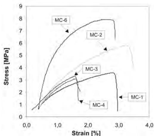
Fig. 5. Stress strain curves for composite magnetic foils
