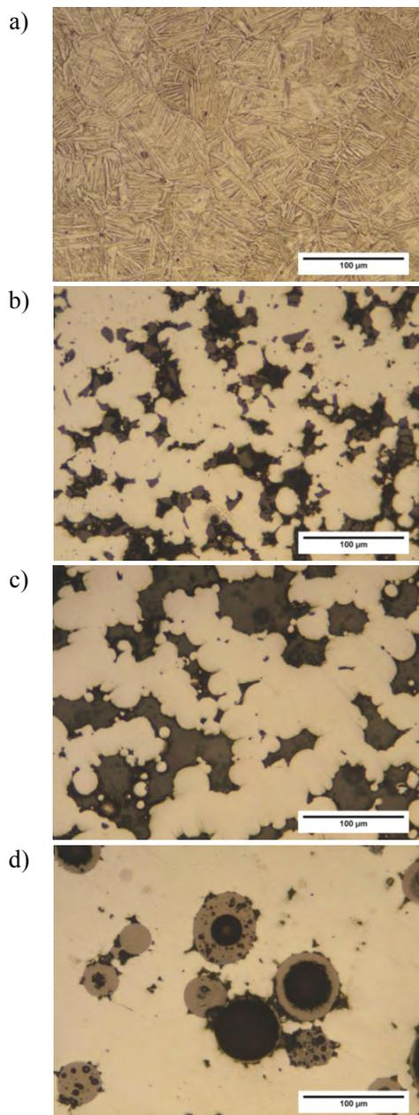
Fig. 1. Microstructure of specimens: a) 100% Ti-6Al-4V, b) 80% Ti-6Al-4V + 20%  $\text{Al}_2\text{O}_3$ , c) 80% Ti-6Al-4V + 20% HAp, d) 80% Ti-6Al-4V + 20% YSZ
