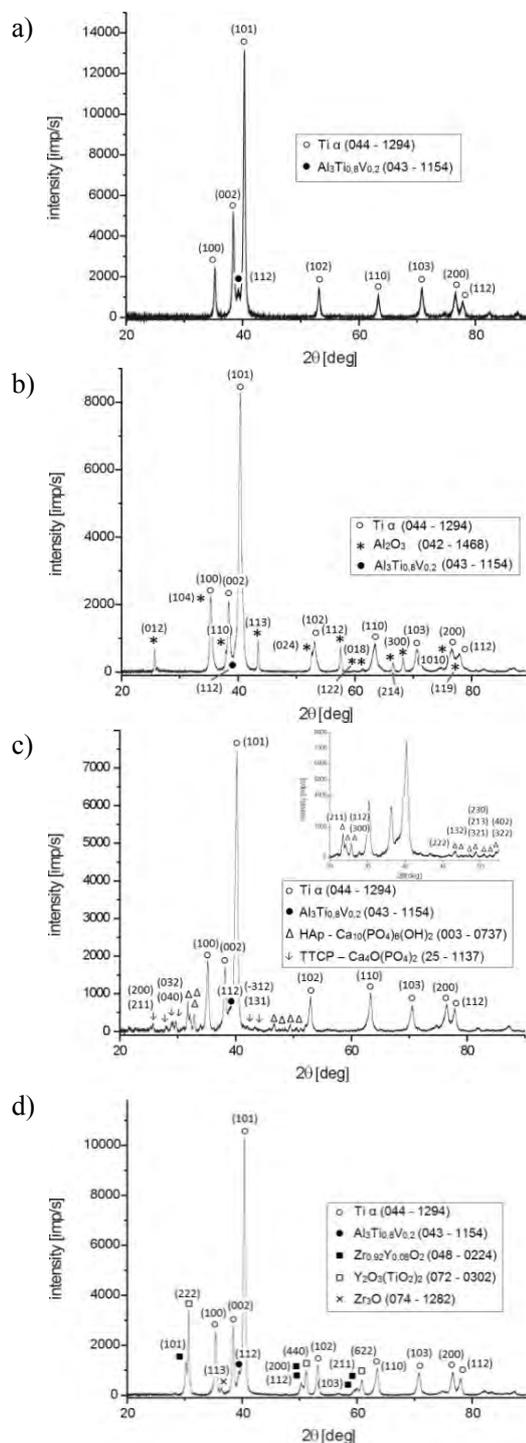
Fig. 2. Diffractograms of specimens: a) 100% Ti-6Al-4V, b) 80% Ti-6Al-4V + 20%  $\text{Al}_2\text{O}_3$ , c) 80% Ti-6Al-4V + 20% HAp, d) 80% Ti-6Al-4V + 20% YSZ
