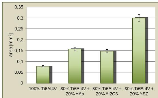
Fig. 6. Wear on surface of individual samples
