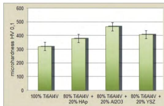
Fig. 4. Microhardness of specimens
