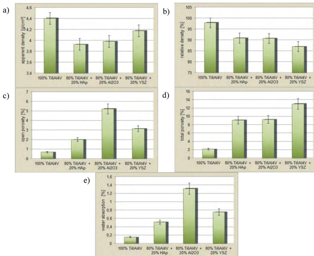
Fig. 3. Graph of: a) apparent density, b) relative density, c) open porosity, d) total porosity, e) water absorption of metallic-ceramic sinters
