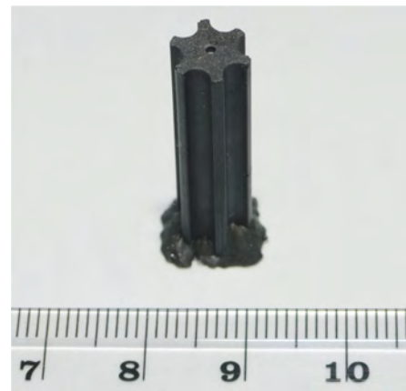
Fig. 1. Centrifugally cast bonded magnet ingot
