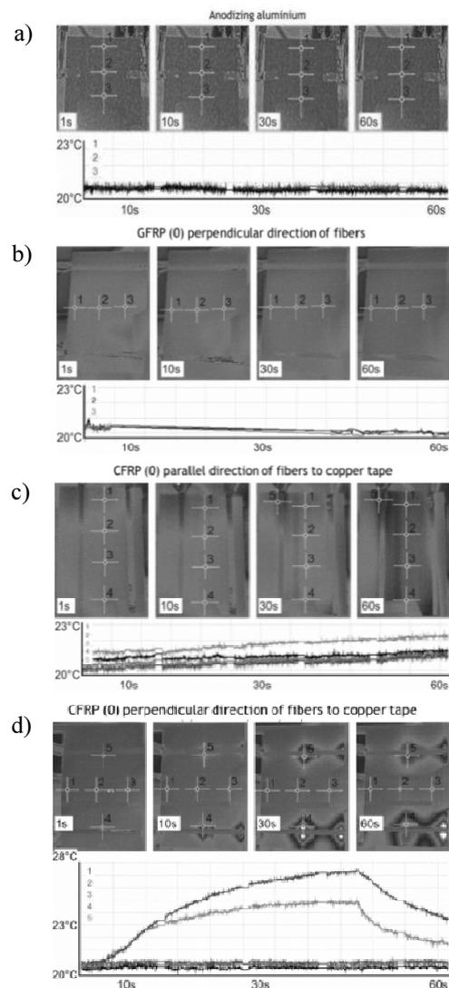
Fig. 4. Views of thermovision camera: a) aluminium alloy with sulphuric anodizing, b) GFRP-R, c) CFRP parallel direction of electrodes to fibres, d) CFRP perpendicular direction of electrodes to fibres
