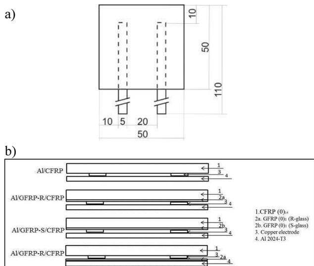
Fig.1. Diagram of laminate and electrode configurations for contact resistivity measurements: a) top view, b) side view
