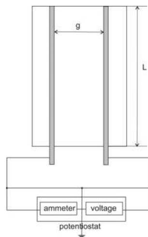
Fig. 2. Connection diagram for surface resistivity measurements; g - distance between electrodes, L - efficiency length of electrode
