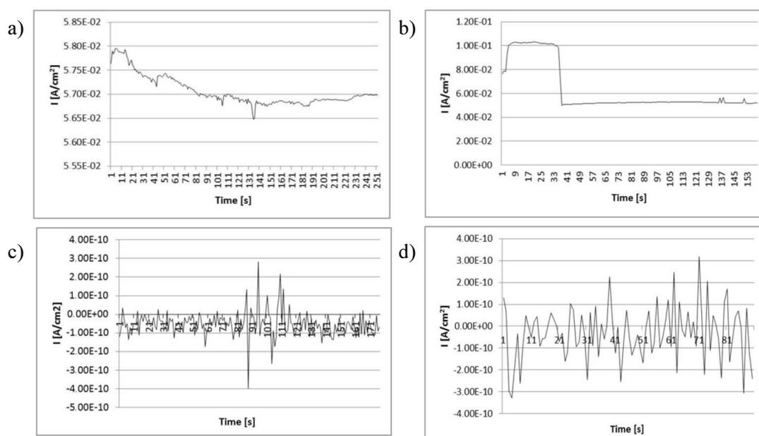
Fig. 5. Curves illustrating surface current density versus time: a) CFRP, electrodes parallel to fibre direction, b) CFRP electrodes perpendicular to fibre direction, c) aluminium anodized in sulphuric acid, d) GFRP-R
