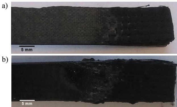
Fig. 5. Photographs of investigated composites CFRP (a) and PANI-EP-CF (b) after burning process
