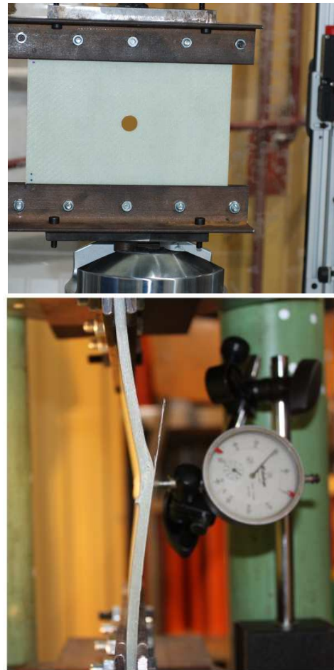
Fig. 4. Experimental testing stand for plates with holes
