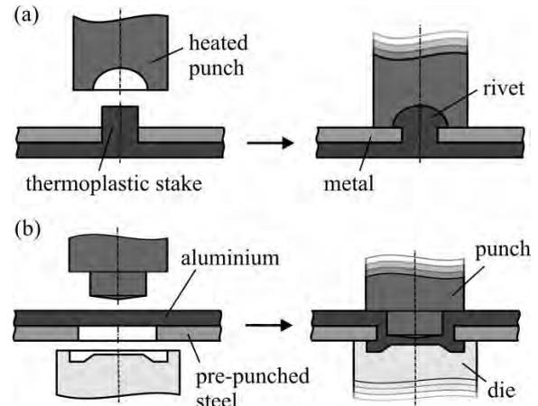
Fig. 1. Schematic illustrations: a) thermoplastic staking process and b) single-staged clinching process with a pre-punched pilot hole
