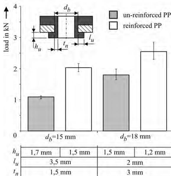
Fig. 4. Dependence of varying main joint dimensions on load bearing capacity of thermoclinching joints with both un-reinforced and reinforced thermoplastic joining partners
