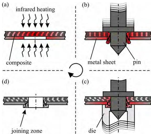
Fig. 2. Schematic illustration of novel thermoclinching process
