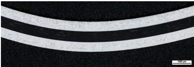
Fig. 2. Panoramic microstructure of aluminum (CAA)-epoxy/glass laminate in [0] configuration after bending test
