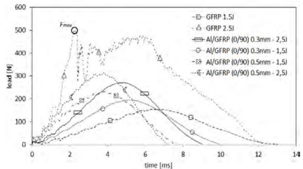
Fig. 1. Experimental load-time curves after impact of Al/GFRP and GFRP laminates
