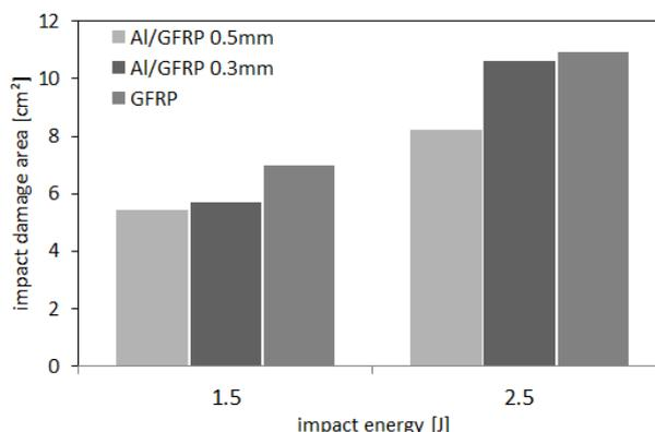
Fig. 3. Value of damage area after low-energy impact of Al/GFRP and GFRP laminates
