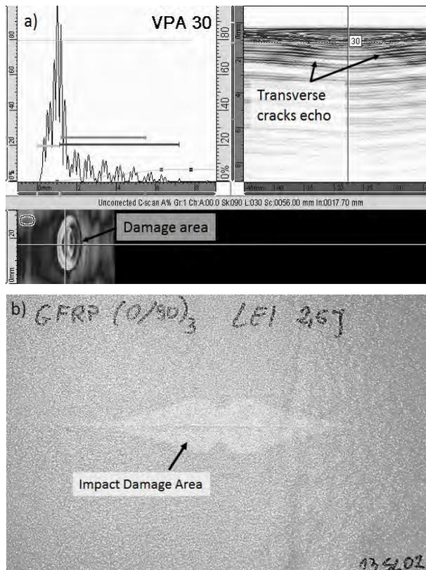
Fig. 2. Damage area of Al/GFRP (ultrasonic view) and GFRP (macroscopic image) after 2.5 J energy impact
