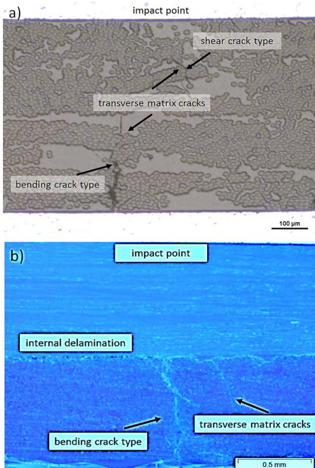
Fig. 5. Examples of laminates failure mechanisms after low-energy impact: Al/GFRP 0.3-2.5 J (a) and GFRP 2.5 J (b)
