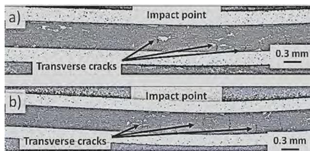
Fig. 4. Cross-sections of Al/GFRP 0.3 mm laminates after low-velocity impact: 1.5 J (a) and 2.5 J (b)
