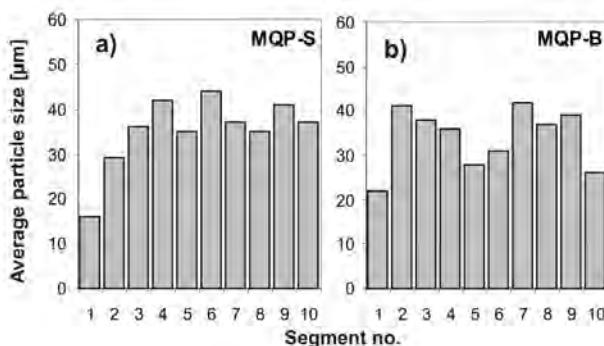
Fig. 8. Variation of average particle size along radius of gear produced with 'spherical' powder (a) and 'flaky' powder (b)
