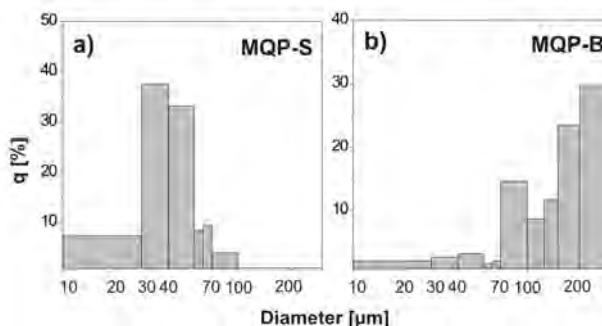
Fig. 3. Particle size distributions in MQP-S powder (a) and MQP-B powder (b)
