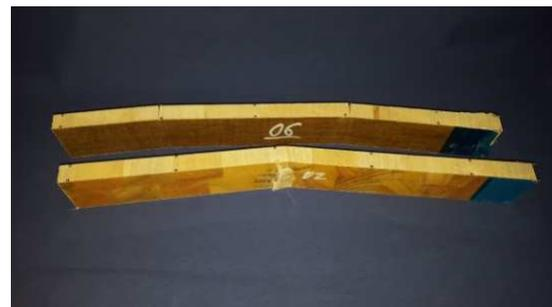
Fig. 5. Sandwich structure samples after 4-point bending test with flax (top) and glass face sheets (bottom)
