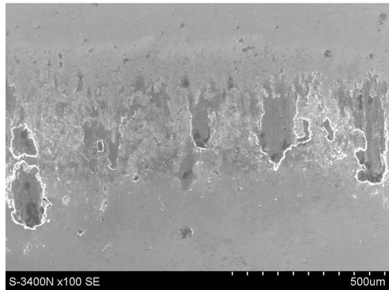
Fig. 7. Surface of steel ball after friction against <200 composite
