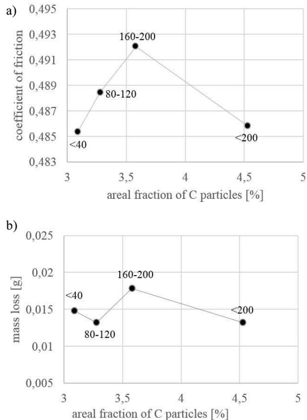
Fig. 4. Influence of C particle presence on composite surface on friction coefficient (a) and mass loss (b)
