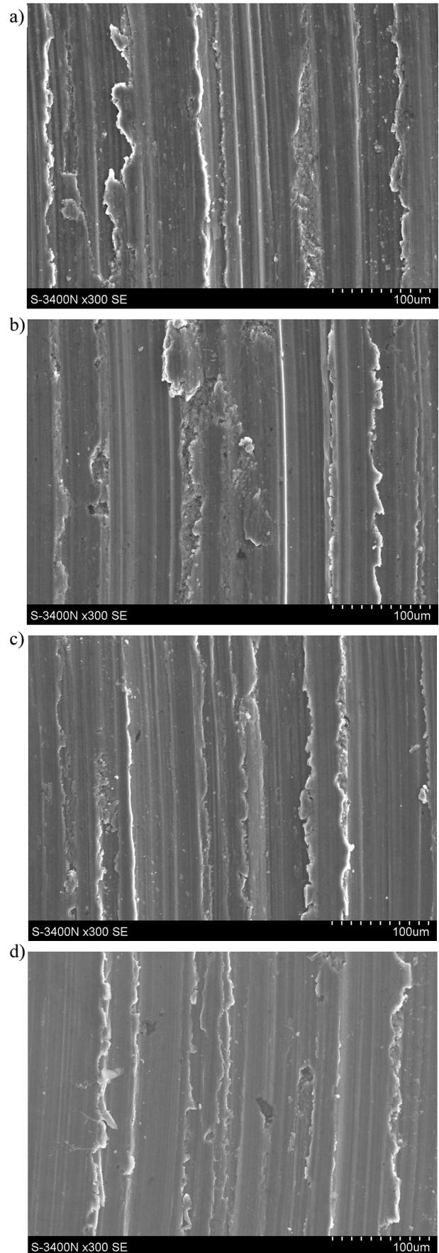
Fig. 6. Surfaces of < 200 (a), < 40 (b), 80÷120 (c), 160÷200 (d) composites after friction against steel ball
