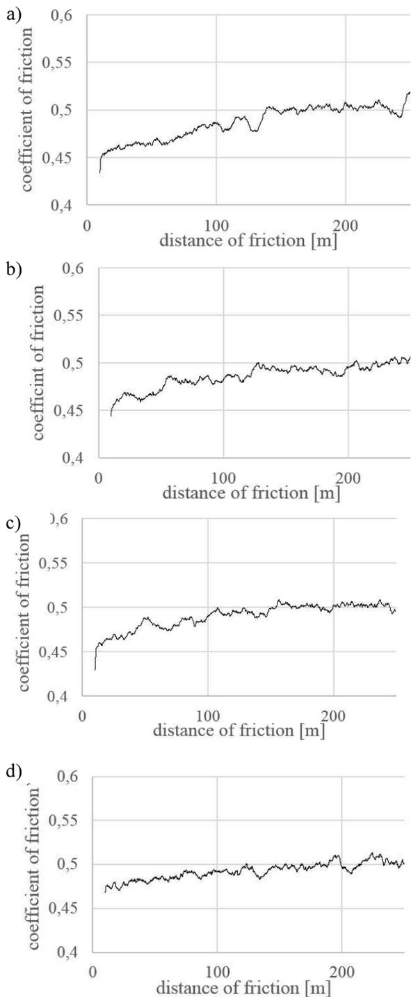
Fig. 5. Variations in friction coefficient on analysed distance for composites: < 200 (a), < 40 (b), 80÷120 (c), 160÷200 (d)
