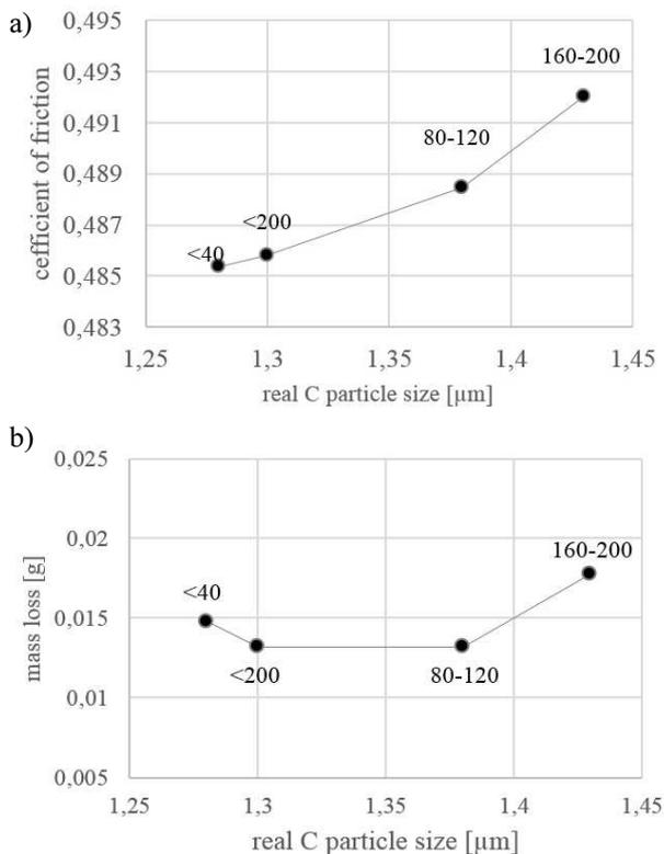
Fig. 2. Influence of real C particle size on friction coefficient (a) and mass loss (b) for Al-Al<sub>2</sub>O<sub>3</sub> composites
