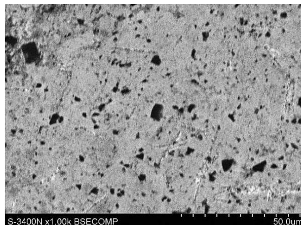
Fig. 1. Example of composite microstructure reinforced by glassy carbon particles
