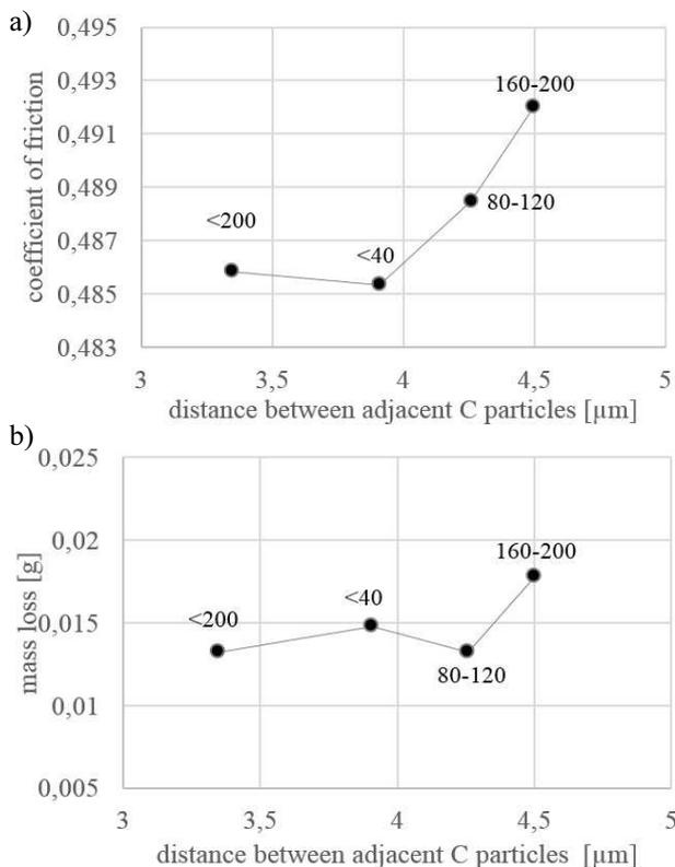
Fig. 3. Influence of average distance between adjacent C particles on friction coefficient (a) and mass loss (b) for Al-Al<sub>2</sub>O<sub>3</sub> composites
