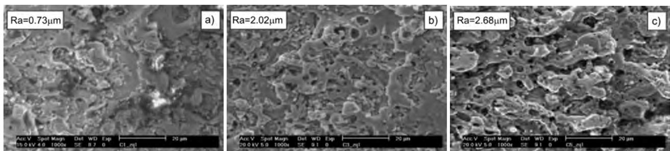
Fig. 2. SEM micrographs of working surfaces of MH13 with 20 vol.% TiC reinforcement, pulse duration and load voltage are: a) 0.5  $\mu\text{s}$ , 122 V; b) 1.5  $\mu\text{s}$ , 122V; c) 2.5  $\mu\text{s}$ , 122 V
