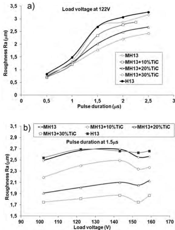
Fig. 3. Surface roughness  $R_a$  as function of: a) pulse duration b) load voltage
