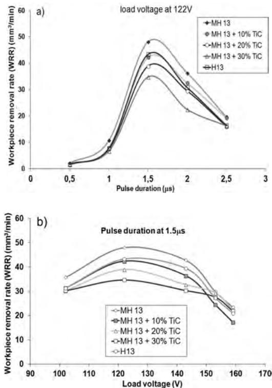
Fig. 1. Workpiece removal rate as function of: a) pulse duration and b) load voltage
