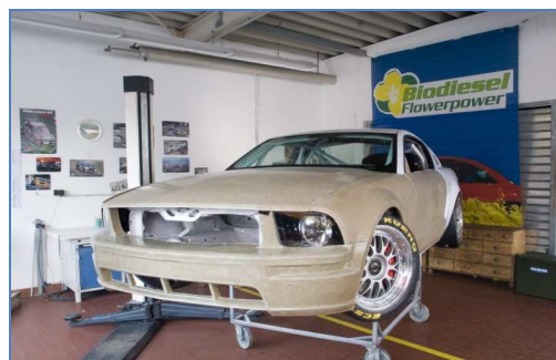
Fig. 5. Bioconcept Ford Mustang car body panels made from natural fibre reinforced bio resin [20]
