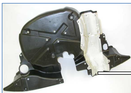
Fig. 7. Under floor protection trim of Mercedes A class made from banana fibre reinforced composites
