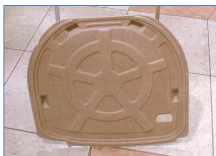
Fig. 4. Spare tire cover made from kenaf fibre reinforced PLA composites for TOYOTA RAUM [16]
