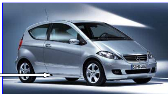
Fig. 7. Under floor protection trim of Mercedes A class made from banana fibre reinforced composites
