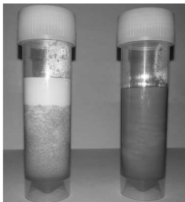
Fig. 5. Sedimentation behaviour of suspension after 48 h: a) \text{Al}_2\text{O}_3 + 10 vol.% Ni, b) \text{Al}_2\text{O}_3 + 20 vol.% Ni
