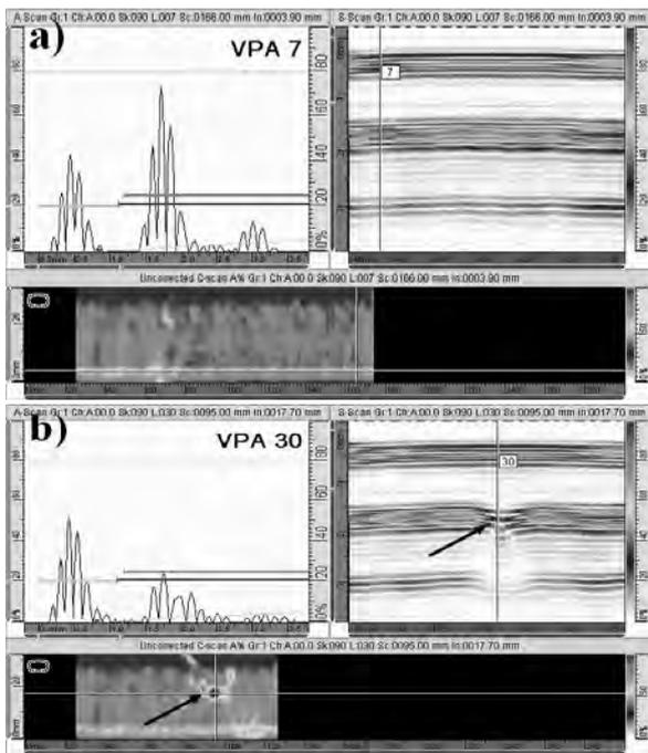
Fig. 3. C-scan views of CFRP after quasi-static indentation equivalent to impact energy 10 J (a) and 25 J (b)
