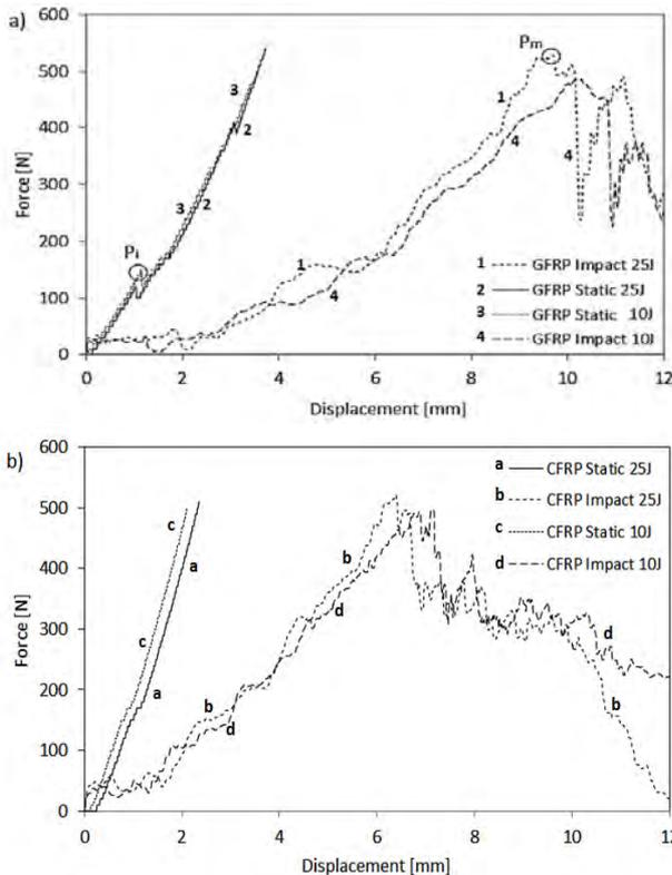
Fig. 1. Typical F-d curves of GFRP (a) and CFRP (b) after low-velocity impact and quasi-static indentation
