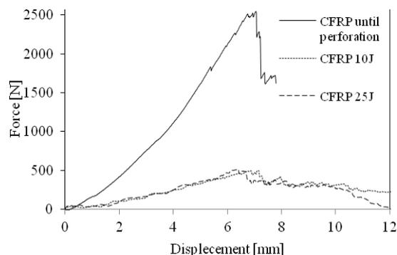
Fig. 5. F-d curve of CFRP laminates representing low-velocity impact and quasi-static indentation until perforation
