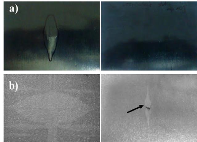
Fig. 2. Macroscopic views of CFRP (a) and GFRP (b) after low-velocity impact 10 J (left) and quasi-static indentation (as 10 J) (right)
