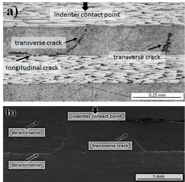
Fig. 4. Cross-section views of CFRP (a) and GFRP (b) laminates after quasi-static indentation as equivalent of 25 J impact energy
