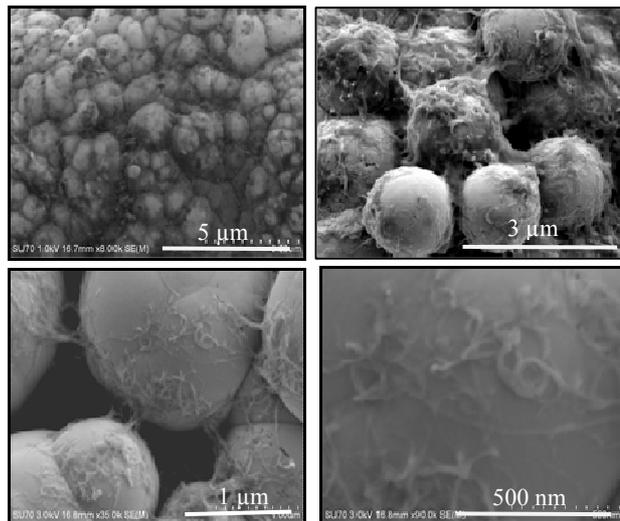
Fig. 5. CNTs in Ni-P/CNT composite layer not fully coated by nickel
