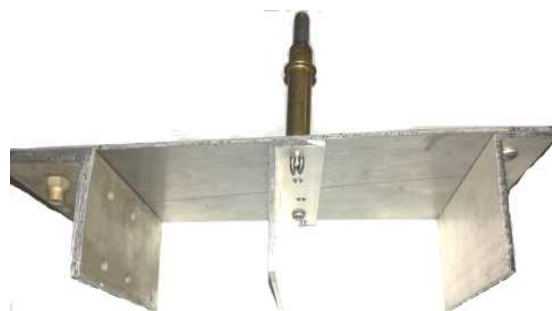
Fig. 3. Mounted joints, construction of ribs and rivets
