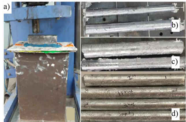
Fig. 3. a) Pouring in mould, b) solidification of molten metal, c) unmoulded cast specimens, and d) finished cast specimens
