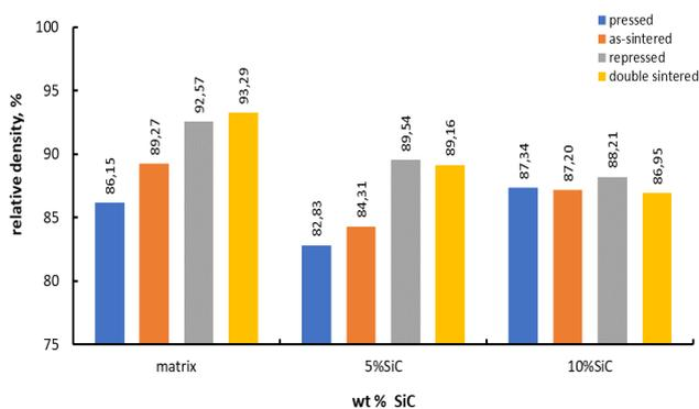
Fig. 3. Influence of different manufacturing steps on density of Al4Cu matrix composites
