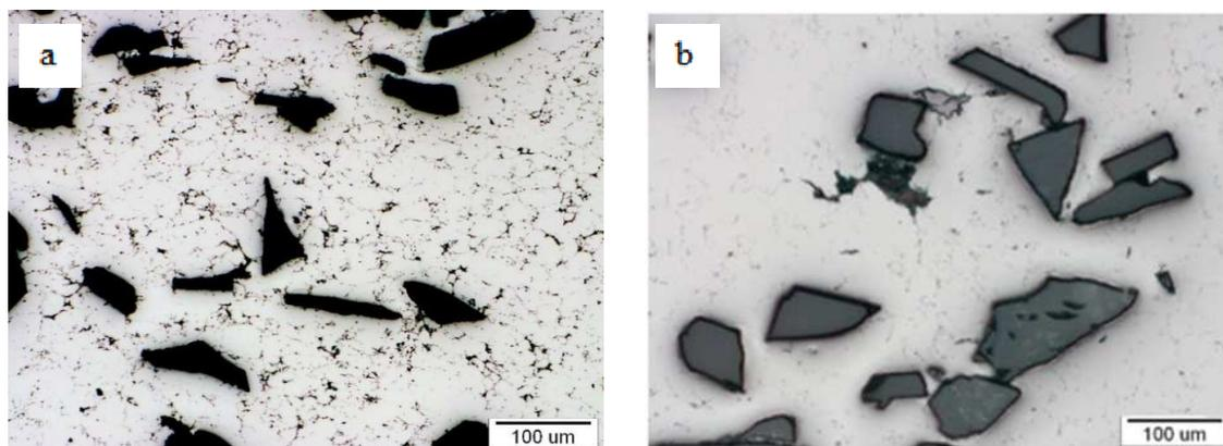
Fig. 9. Microstructure of Al + 10 wt.% SiC composite
