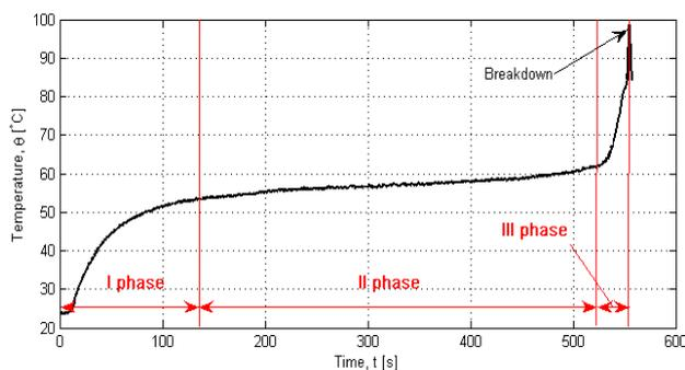
Fig. 2. Typical temperature evolution during thermal fatigue
