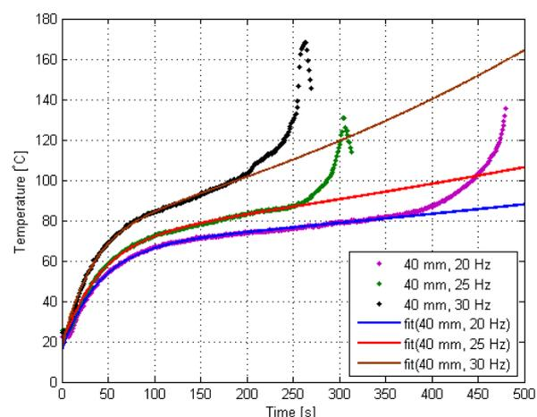
Fig. 4. Exemplary results of fitting for different cases of excitation frequency
