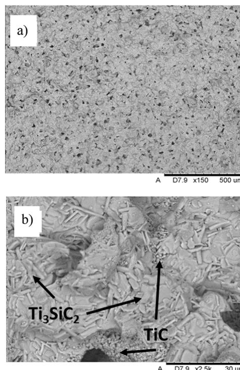
Fig. 3. Overall porosity of manufactured material after SHS (a), Ti<sub>3</sub>SiC<sub>2</sub> microstructure with round TiC inclusions (b)
