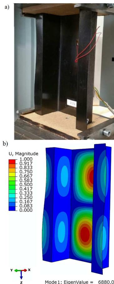
Fig. 5. Stability loss of composite profile under compression: a) EXP, b) FEM
