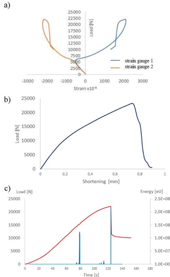
Fig. 9. Failure characteristics: a) strain measurement, b) FEM analysis, c) acoustic emission measurement
