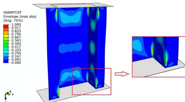
Fig. 6. Damage initiation in composite profile - HSNMTCRT tensile matrix damage
