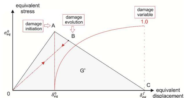
Fig. 3. Damage initiation and evolution law
