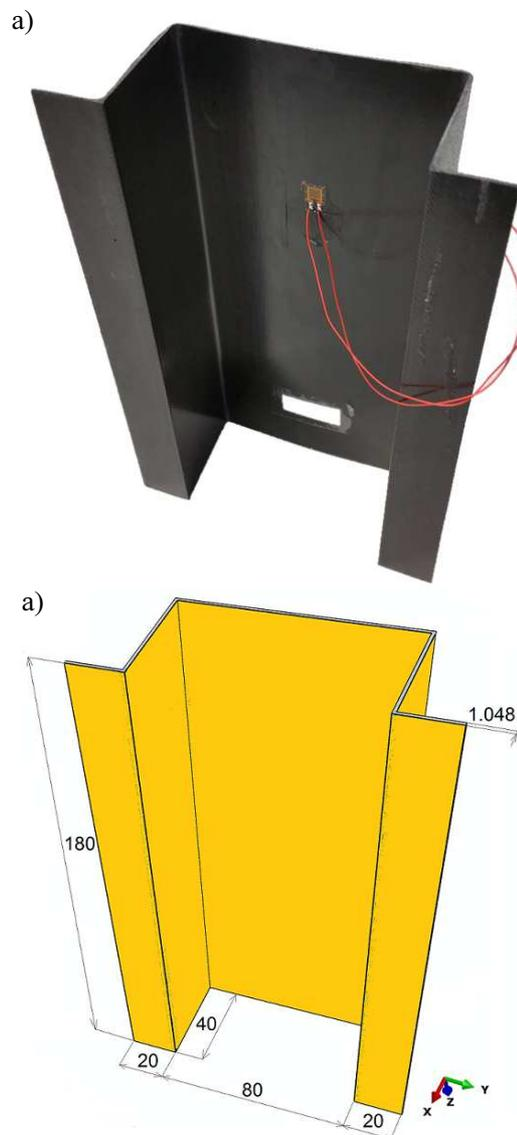
Fig. 1. Composite profile with open cross-section: a) physical model, b) geometric model
