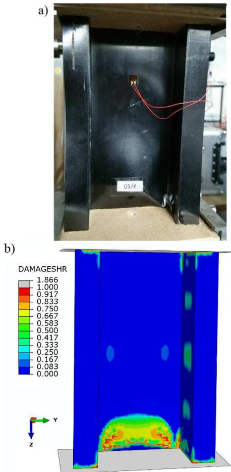
Fig. 8. Loss of load capacity in composite profile - whole model: a) EXP, b) FEM (shear damage)
