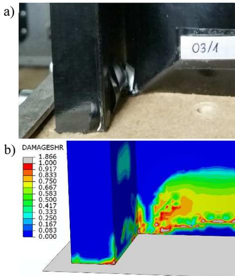
Fig. 7. Loss of load capacity in composite profile: a) EXP, b) FEM (shear damage)
