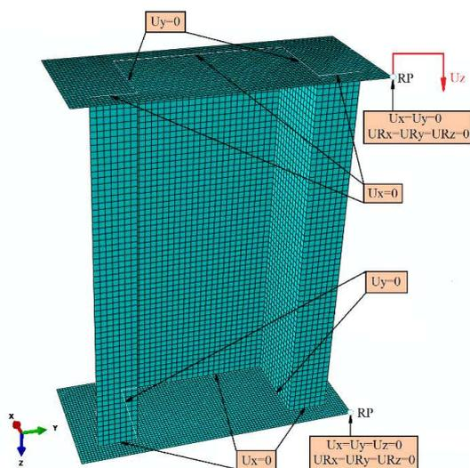
Fig. 4. Boundary conditions of numerical model
