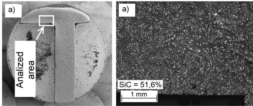
Fig. 6. Distribution of particles in running gate of  $\phi 6$  mm casting filled using centrifugal method: a) location of analyzed area, b) microstructure
