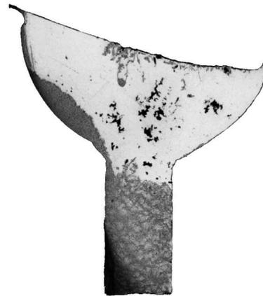
Fig. 8. Micrographs of gating system with visible reinforcement-matrix interface
